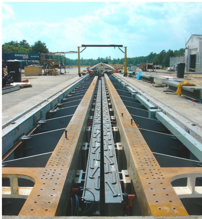
Fig. 30: General Atomics full scale maglev test track [47]
