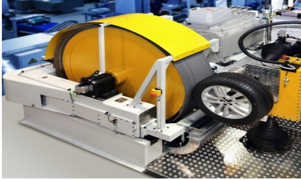
Figure 2.2: Drum Type TTM. [14]
