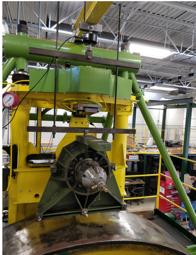
Figure 3.2: Z-axis Load Cell Calibration Jig
