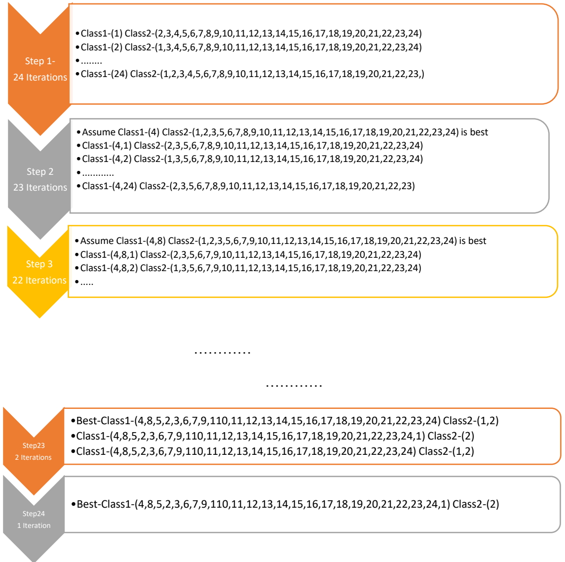
Figure 4. 3: Process flow of Modified Heuristic Algorithm 2 (Heuristic Algorithm 3)
