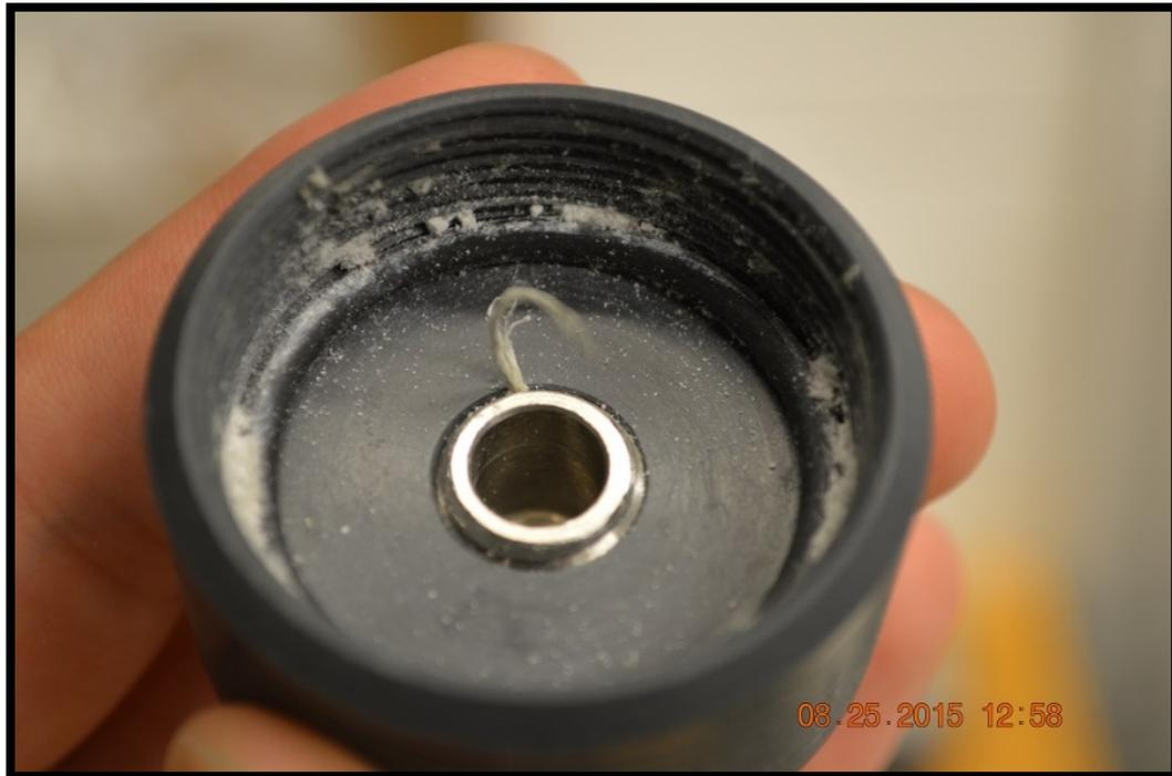
Figure 3.6. Desiccant holder cap after testing
