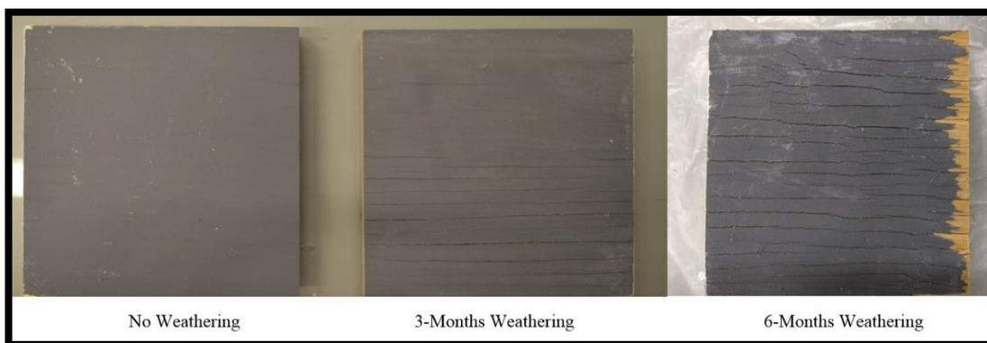
Figure 4.2. Visible weathering effects on coating B
