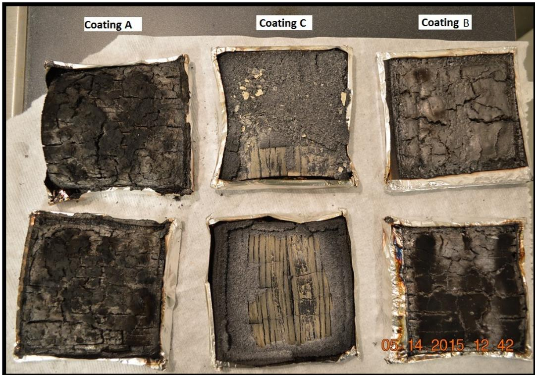
Figure 4.33. Comparison of the specimens at the end of the fire test
