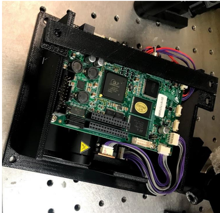
FIGURE 3. 4: Projector inside the 3-D printed Housing
