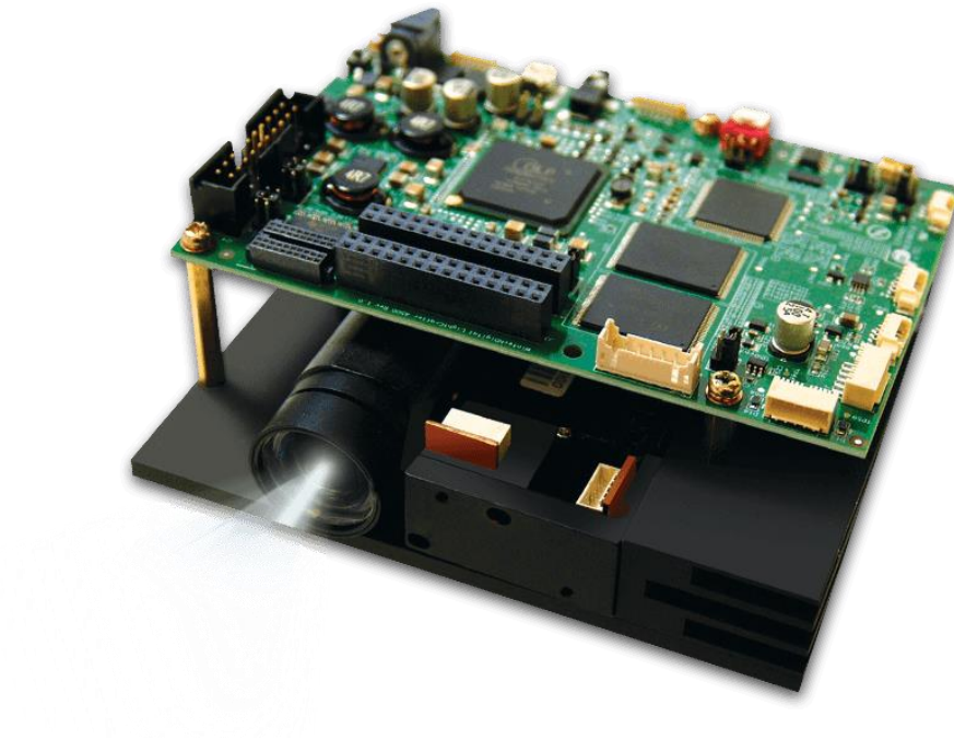
FIGURE 3. 2: DLP Light crafter 4500 with all components intact
