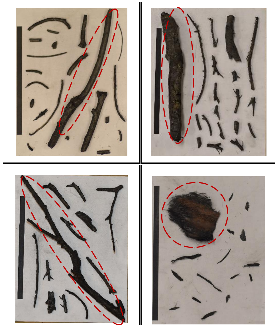
Figure 4.16. Various Shape, Size, and Mass of Firebrands Collected from Generation Experiments of Three Vegetation Species
