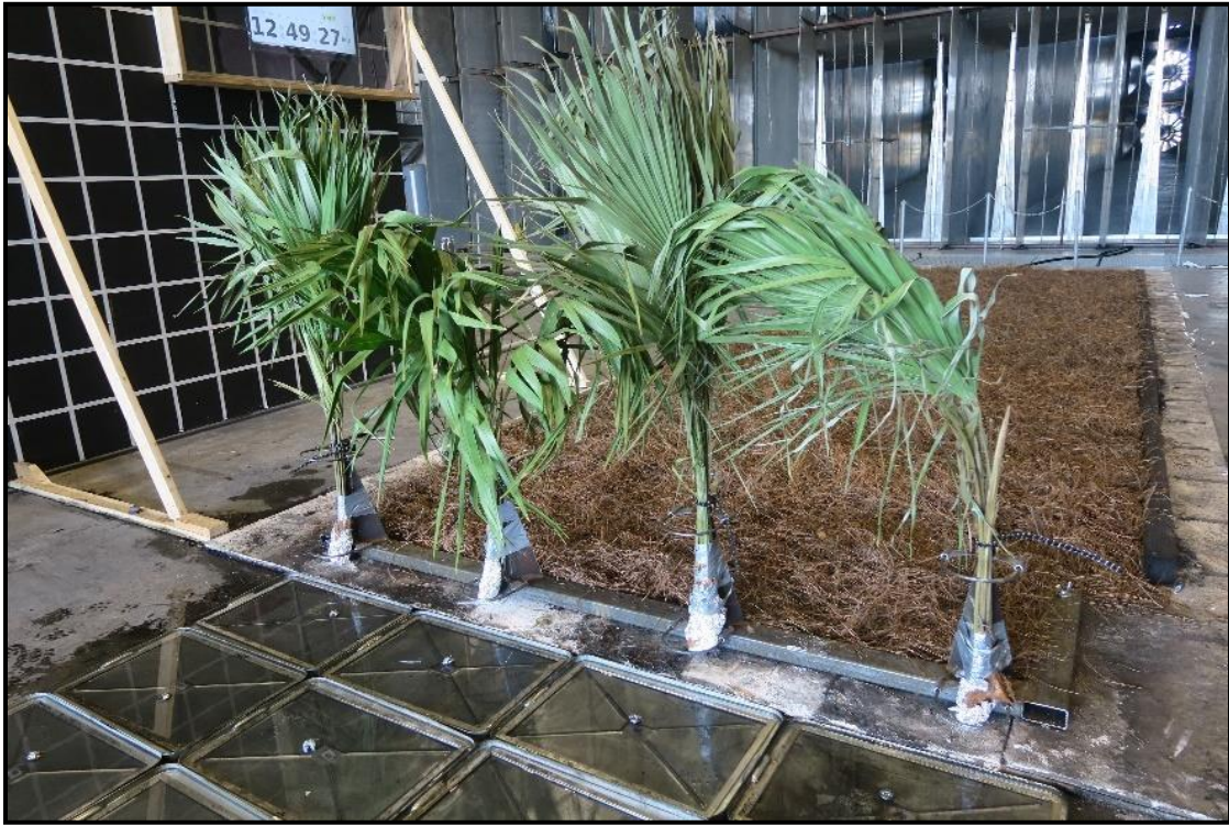
Figure 3.5. Pine Needle Bed and Saw Palmetto Samples before Test (Photo Courtesy of IBHS)
