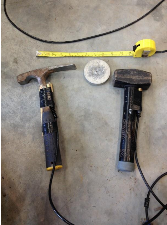
a.) Hammers used for MASW
