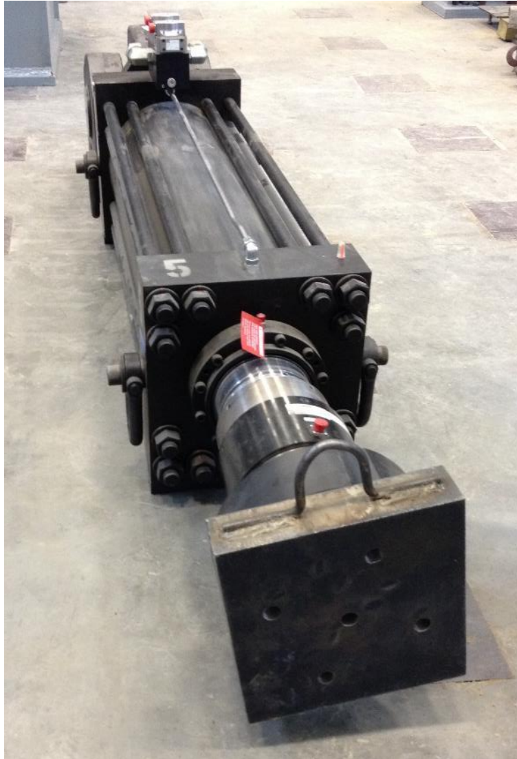
Figure 3-15. Load actuator used for static axial pile load testing at UNCC geotechnical test pit
