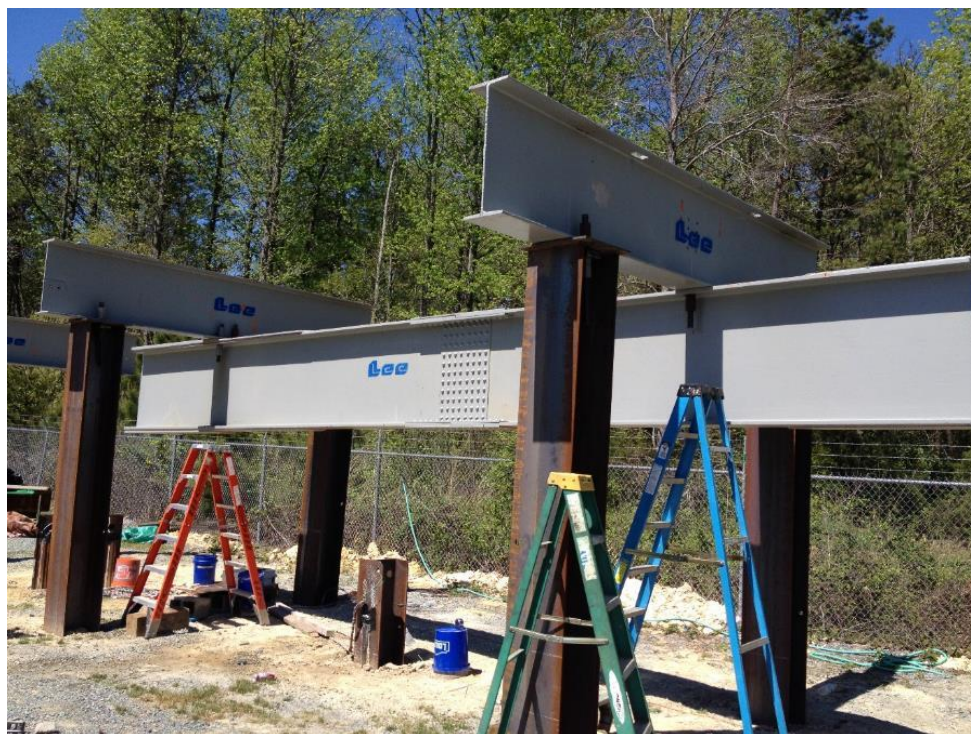
Figure 4-19. Image of reaction frame used for static axial load tests
