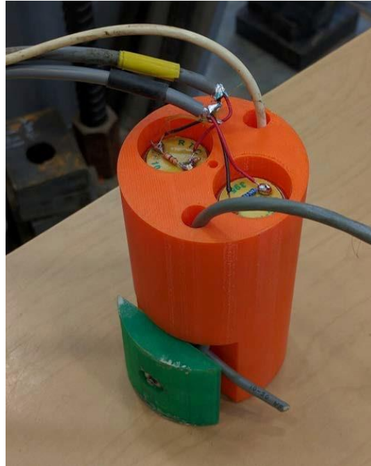
a.) 3D printed sensor casing for crosshole test
