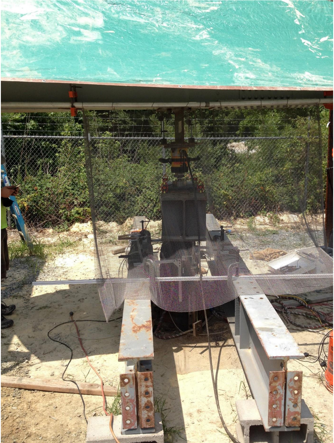
Figure C-19. Image of static load test setup for sheet pile at ICE field site
