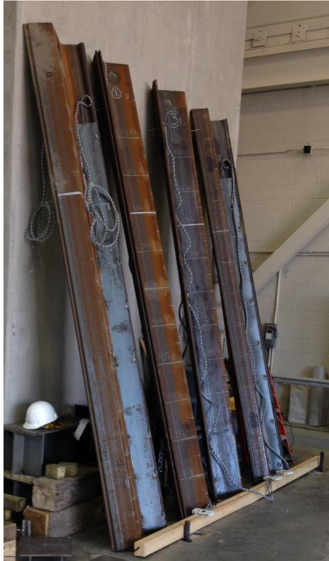
Figure 3-10. Image of instrumented sheet piles ready for installation at UNCC geotechnical test pit
