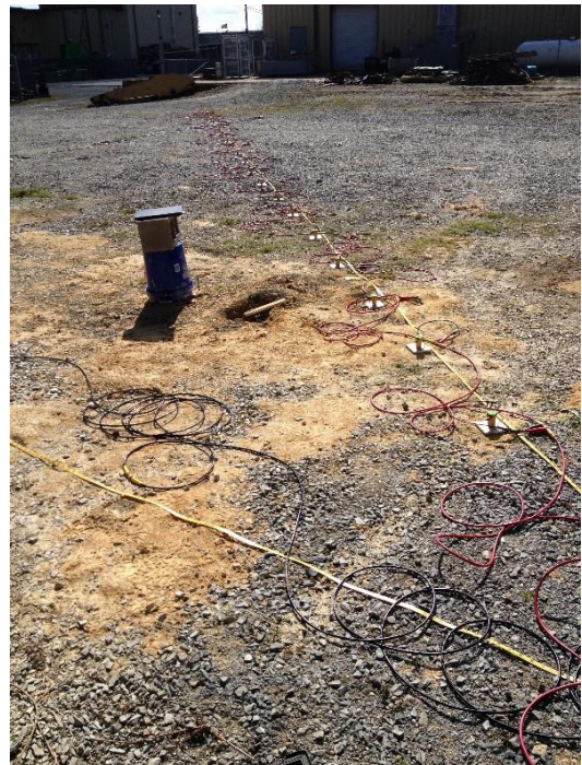
d.) Additional array for MASW testing
