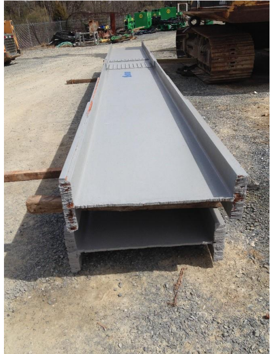
b.) Beams for reaction frame, provided by Lee Construction Company
