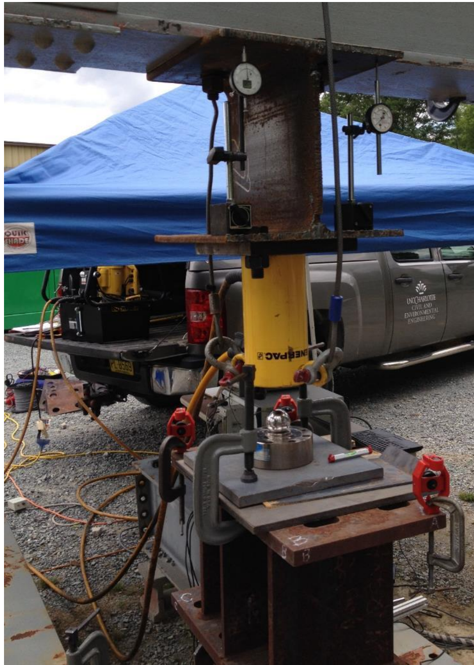
Figure 4-20. Image of H-pile field load test
