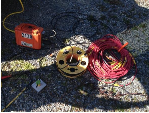
a.) MASW equipment
