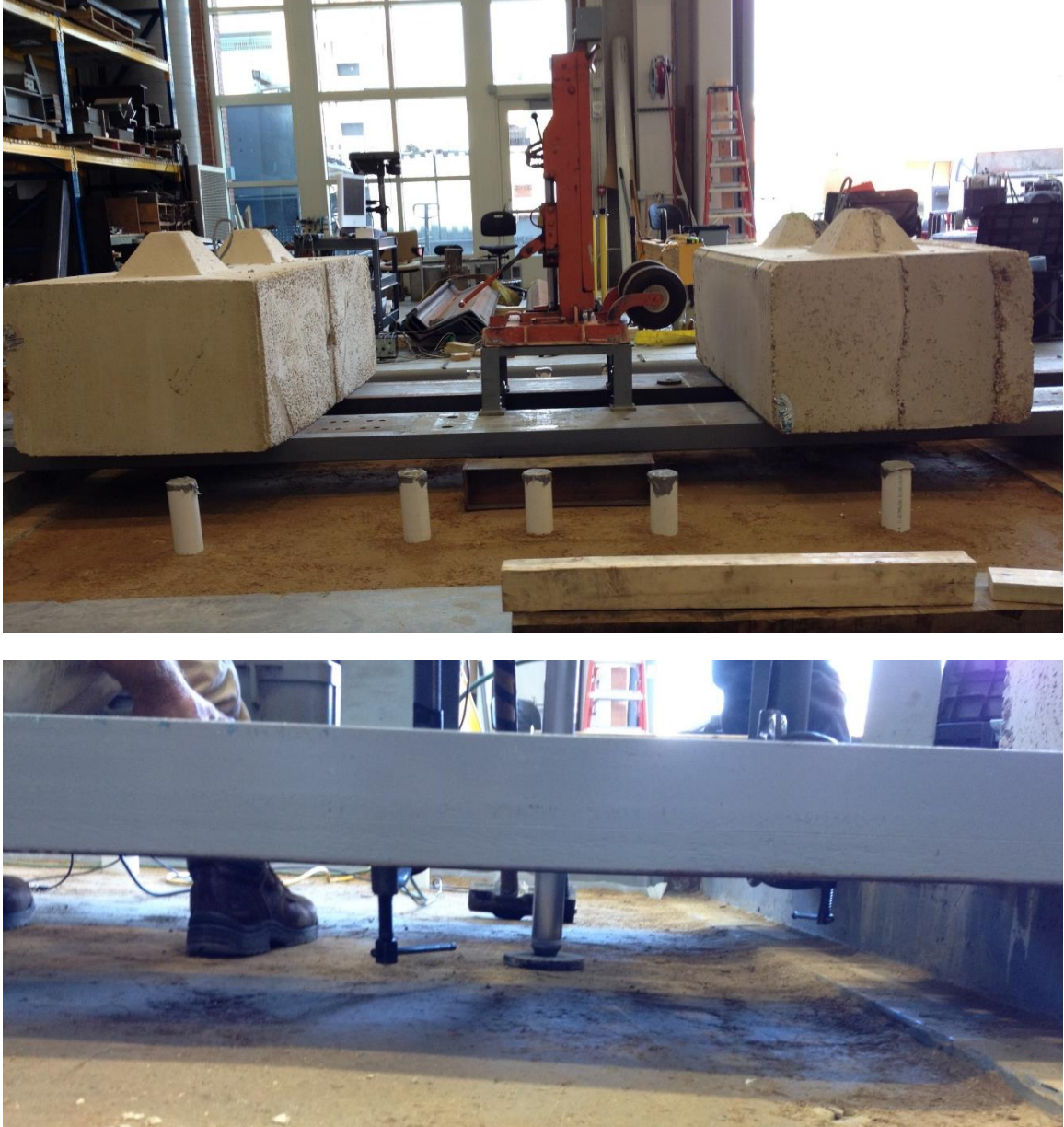
Figure B-7. Images of test setup used for SCPTu testing of EPIC geotechnical test pit performed by S&ME (Charleston, SC, office)
