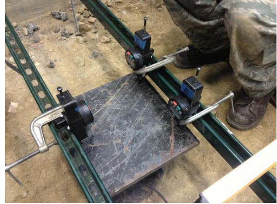
(b) Dial gauges for plate load test
