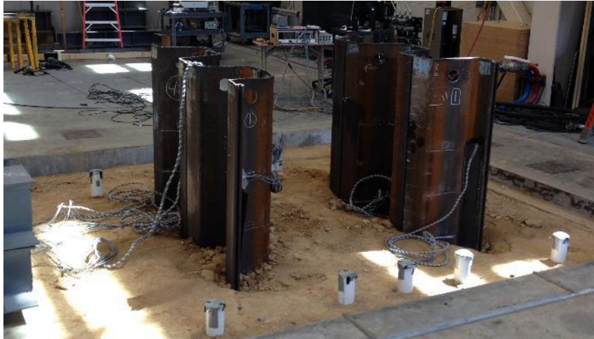
Figure 3-14. Image of pile walls after driving at UNCC geotechnical test pit
