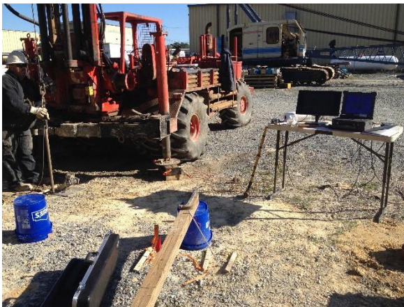
a.) CME 550X rig used for pushing SCPTu cone and rods
