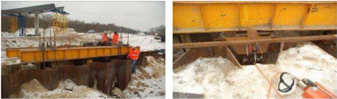
Figure 2-21. Sheet pile test setup (from Skyline Steel LLC 2009)
