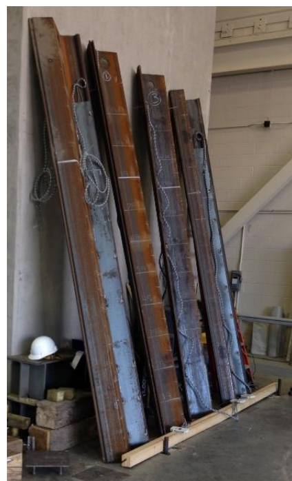
d.) Instrumented sheet piles
