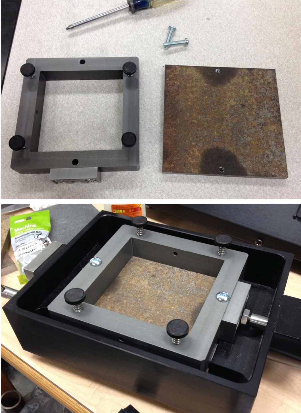
Figure B-17. Images of interface shear test setup, above: steel coupon, top half of shear box, below: assembled box
