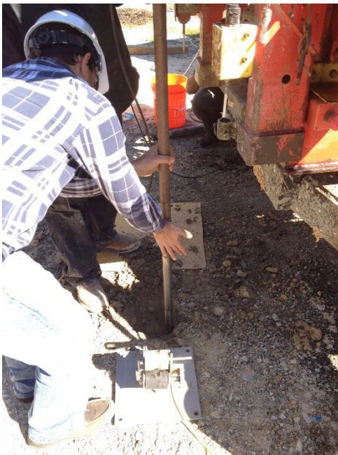
c.) Placing SCPTu cone prior to sounding
