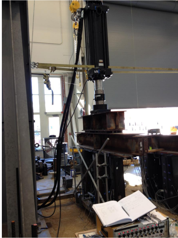
Figure 3-16. Image of static axial pile load test setup at UNCC geotechnical test pit
