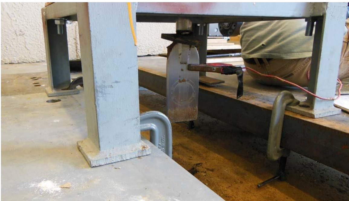
Figure B-8. Image of DMT testing at EPIC geotechnical test pit prior to sheet pile installation
