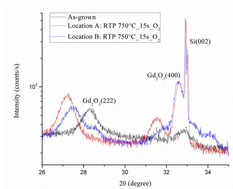
Figure 21. XRD patterns of the 60 nm-thick  $Gd_2O_3$  deposited on n-type Si(100) at  $175^\circ C$ , before and after RTP at different location.
