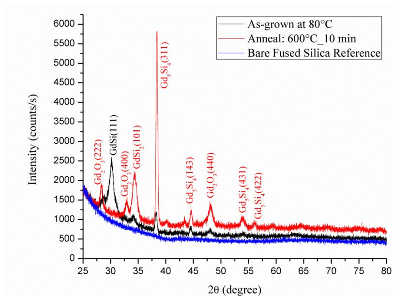
Figure 22. XRD patterns of an 80 nm-thick  $\text{Gd}_2\text{O}_3$  deposited on fused silica substrate at  $200^\circ\text{C}$  before and after annealing in furnace with  $\text{N}_2$  ambient
