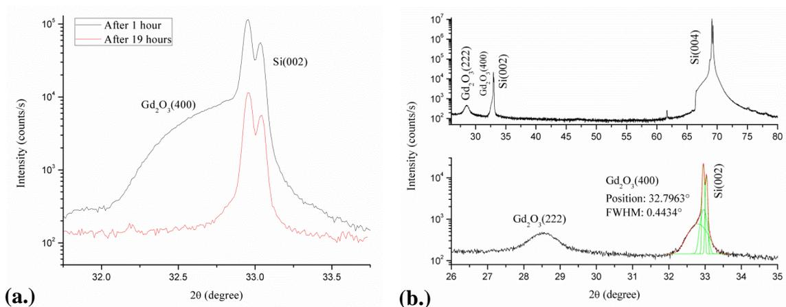
Figure 19. XRD pattern illustrating (a) the instability of the 30 nm-thick  $Gd_2O_3(100)$  grown on the intrinsic Si(100) substrate through the disappearance of the  $Gd_2O_3(400)$  peak over a course of 19 hours, and (b) a stable  $Gd_2O_3(100)$  on i-Si(100) with a lower crystalline quality.
