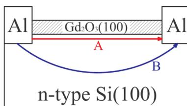
Figure 26. Schematic diagram showing possible conduction paths between two electrodes
