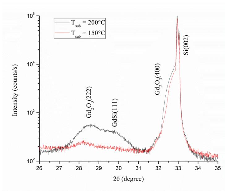
Figure 20. XRD patterns of the polycrystal with predominant  $\text{Gd}_2\text{O}_3(100)$  structure grown on the intrinsic  $\text{Si}(100)$  illustrating the suppression of the silicide formation through a low growth temperature.
