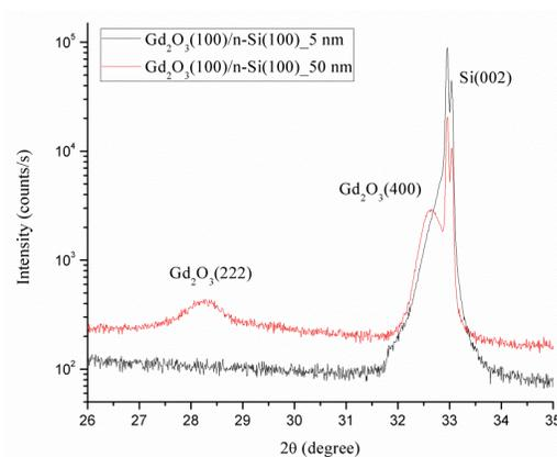
Figure 16. XRD pattern of the growths on n-type Si(100) comparing a single crystal  $\text{Gd}_2\text{O}_3(100)$  and the polycrystal with a predominant  $\text{Gd}_2\text{O}_3(100)$  structure. The thicknesses for each sample are 5 and 50 nm, respectively.
