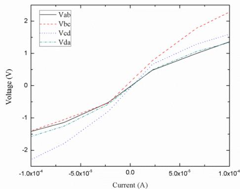
Figure 33. IV curve showing a decent ohmic characteristic between the four Al contacts on n-type substrate with the  $Gd_2O_3(110)$  deposited on top
