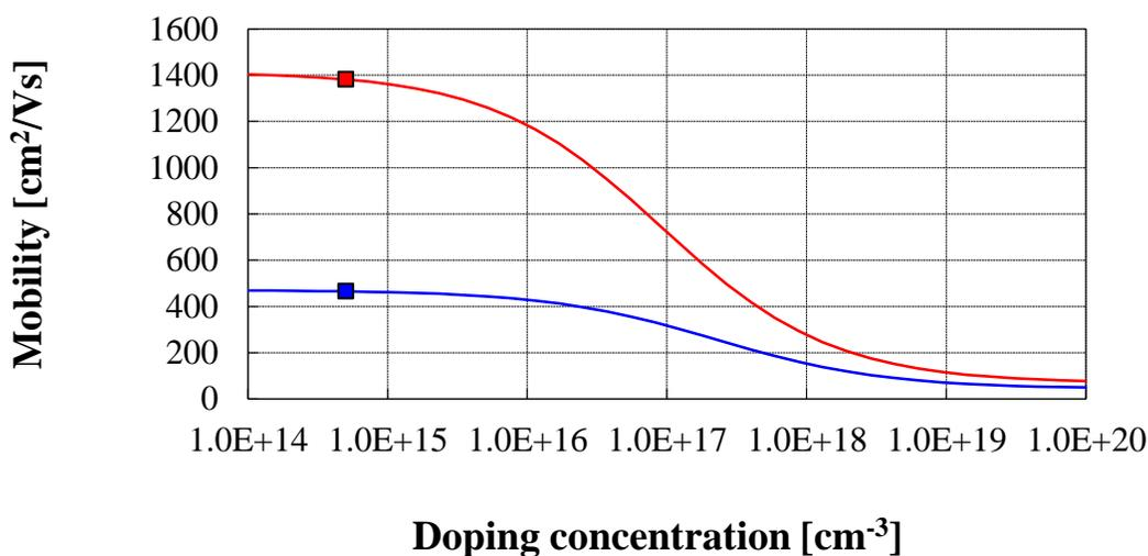
Figure. 23 Variation of carrier mobility in bulk silicon at 300K with doping concentration
