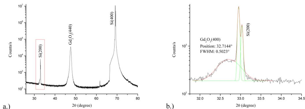
Figure 32. XRD pattern illustrating the polycrystalline structure with  $Gd_2O_3(110)$  and  $Gd_2O_3(100)$  grown on n-type Si(100). a.) Full scan, b.) Enlargement of the red box
