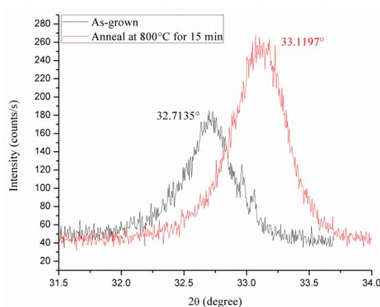
Figure 18. XRD pattern illustrating the strain relaxation of the 150nm-thick  $\text{Gd}_2\text{O}_3(100)$  grown on p-type Si(100) after the annealing at  $800^\circ\text{C}$  for 15 min
