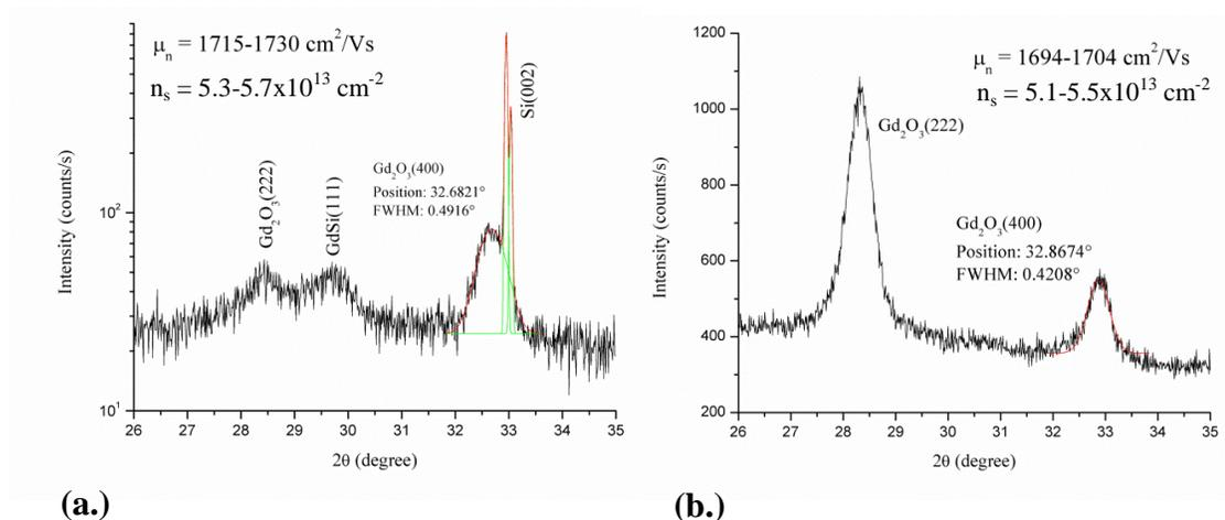
Figure 28. Degradation of Hall mobility due to different structural composition of the (a.) 90-nm and (b.) 80-nm thick polycrystalline  $\text{Gd}_2\text{O}_3$  grown on the n-type substrate
