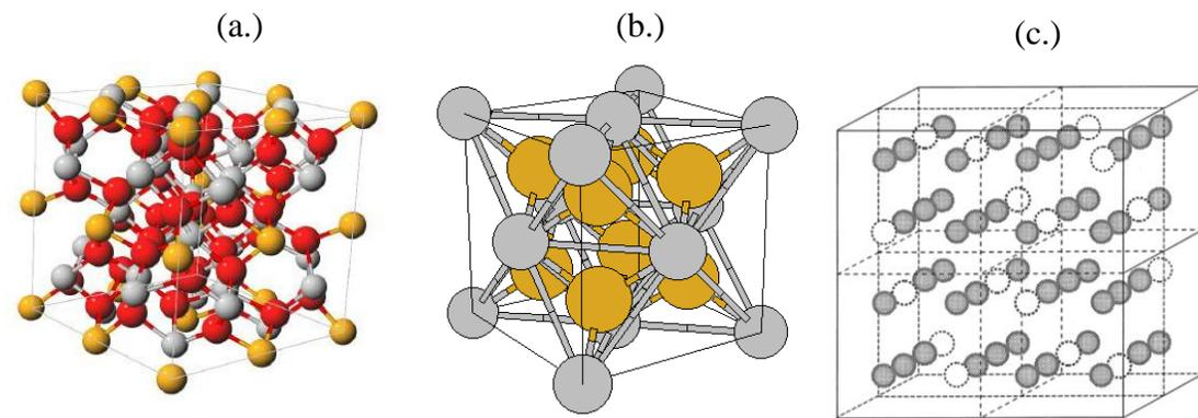
Figure 6. Illustration of (a.) cubic bixbyite structure [Gray =  $Gd^{3+}$ , Red =  $O^{2-}$ , Yellow = surface  $Gd^{3+}$ ], (b.) fluorite structure [Gray = cation ( $Ce^{2+}$  or  $Ca^{2+}$ ), Yellow = anion ( $O^{2-}$  or  $F^{2-}$ )], and (c.) positions of oxygen (gray sphere) and oxygen vacancies (hollow sphere) within the cubic bixbyite unit cell [39-41]
