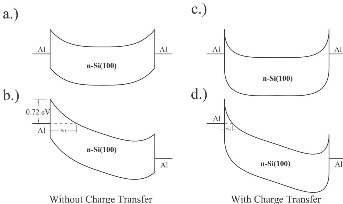
Figure 25. Interface Band diagrams between two Al contacts without the charge transfer (a, b) and with the charge transfer (c, d) at equilibrium and with applied bias.
