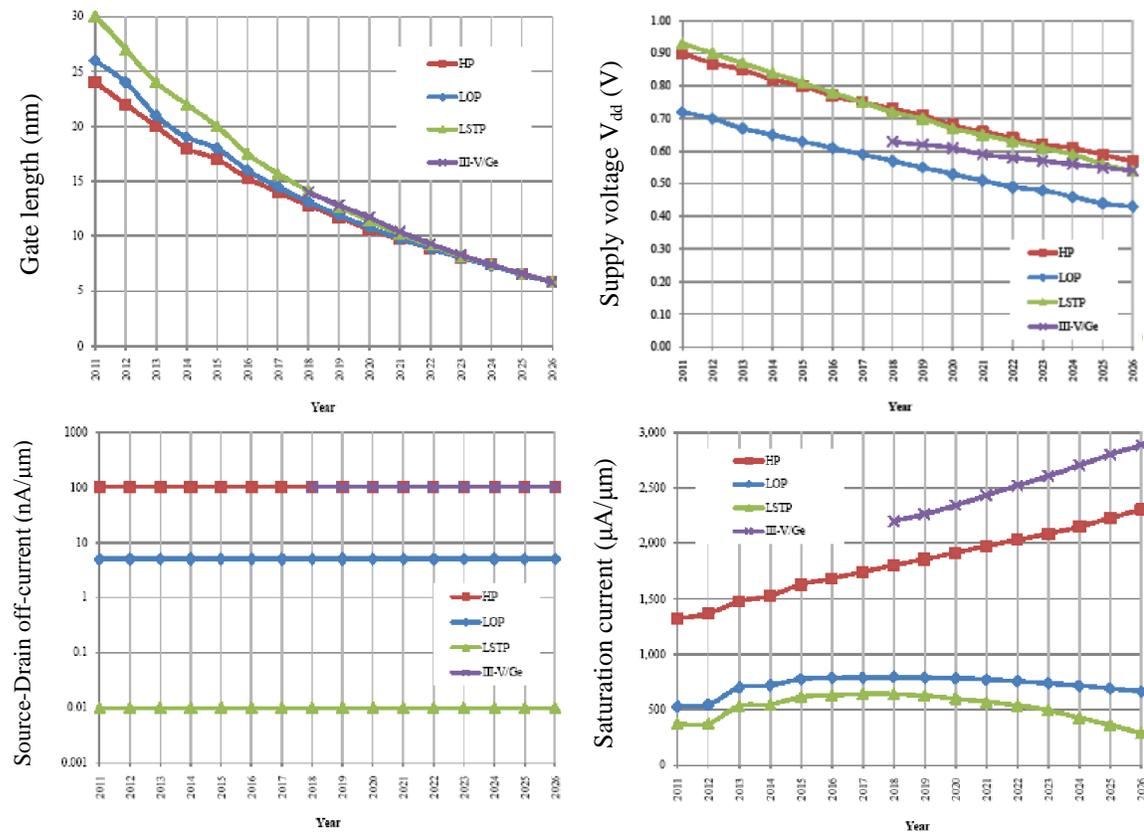
Figure 4. ITRS 2011 scaling trend of logic technologies with year; (a.) Gate length, (b.) Supply voltage, (c.) Off-current, (d.) Saturation on-current. (HP = High Performance, LOP = Low Operating Power, LSTP = Low Standby Power) [7]
