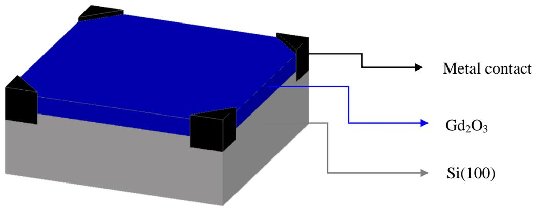
Figure 14. Van der Pauw configuration for Hall measurement
