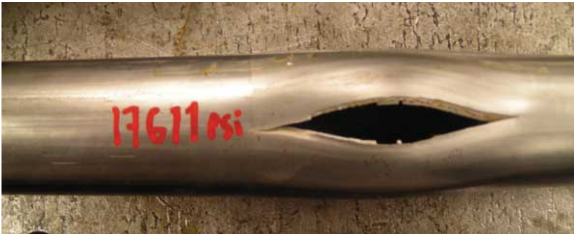
Figure 1.1: Hoop stress failure [2]
