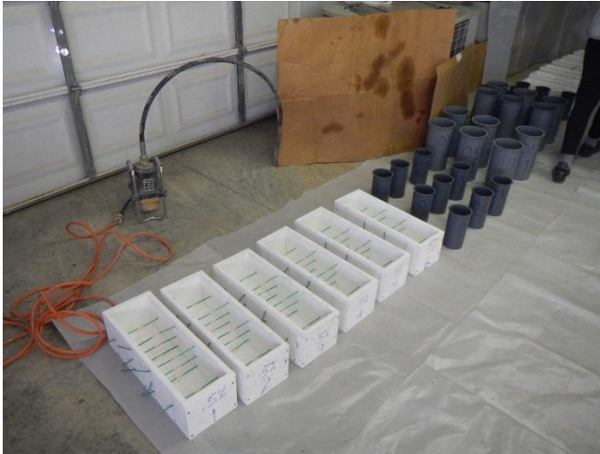
FIGURE 2: Formwork for making self-sensing concrete
