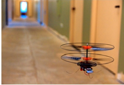
Figure 2.6: SensorFly node flying in a hallway [21]
