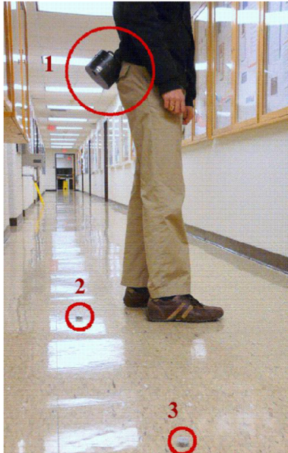
Figure 2.3: Automatic breadcrumb system working, using a dispenser (1) and breadcrumbs (2 and 3) [15]
