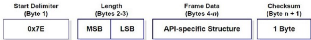
Figure 3.6: API 1 Frame Structure [34]
