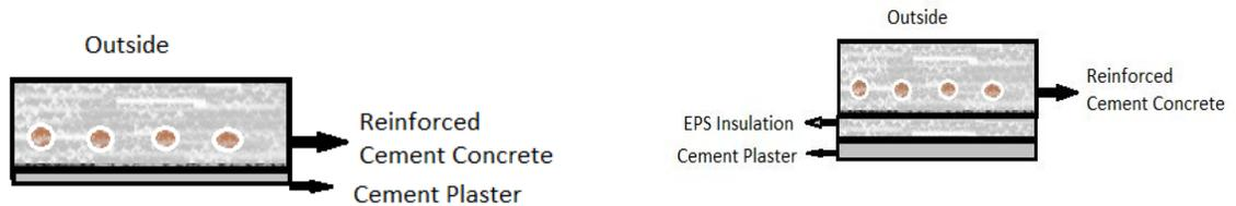
FIGURE 19: Roof construction for reference building and its TRNSYS representation (Right)
