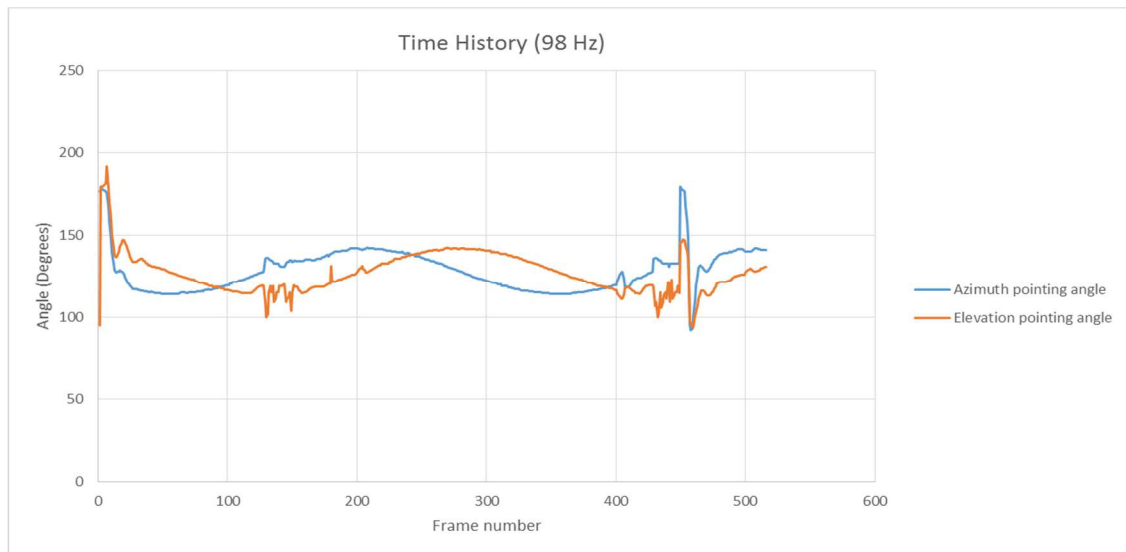
Figure 3: Time history of the fixed frame rate sensor at 98Hz laser modulation
