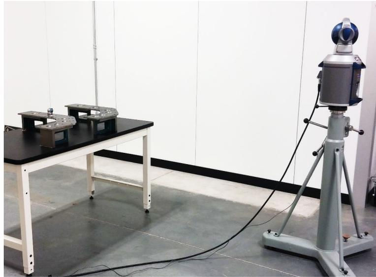
Figure 20. Measurement of the outer profile with a FARO ION laser tracker
