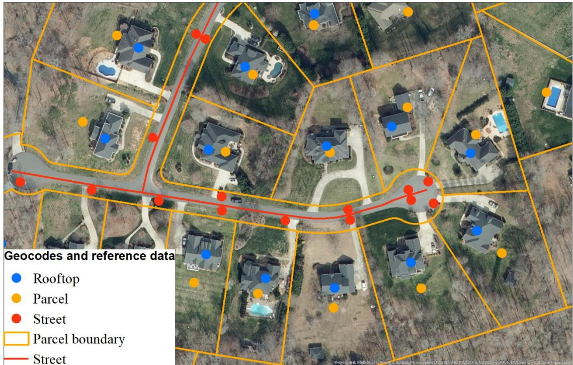
Figure 1.4: The 3 types of reference datasets: rooftop centroid in blue (most accurate), parcel centroid (reasonably accurate) and street centerline (less accurate)
