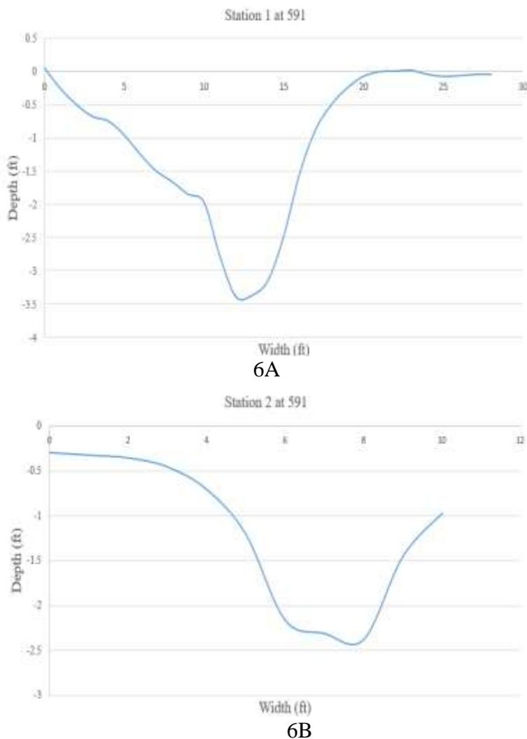
**Figure 6 (A and B): Cross Section of Channel for Site 1 (591)**
