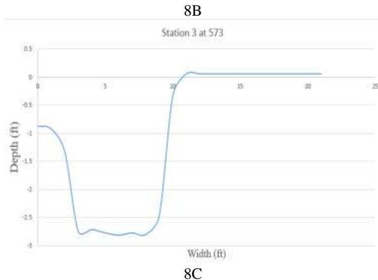
**Figure 8 (A, B, C): Cross Section for Channel for Site 2 (573)**
