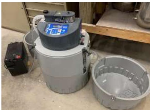
**Figure 9: ISCO 6712 Sampler with 730 Flow Bubbler Module**
