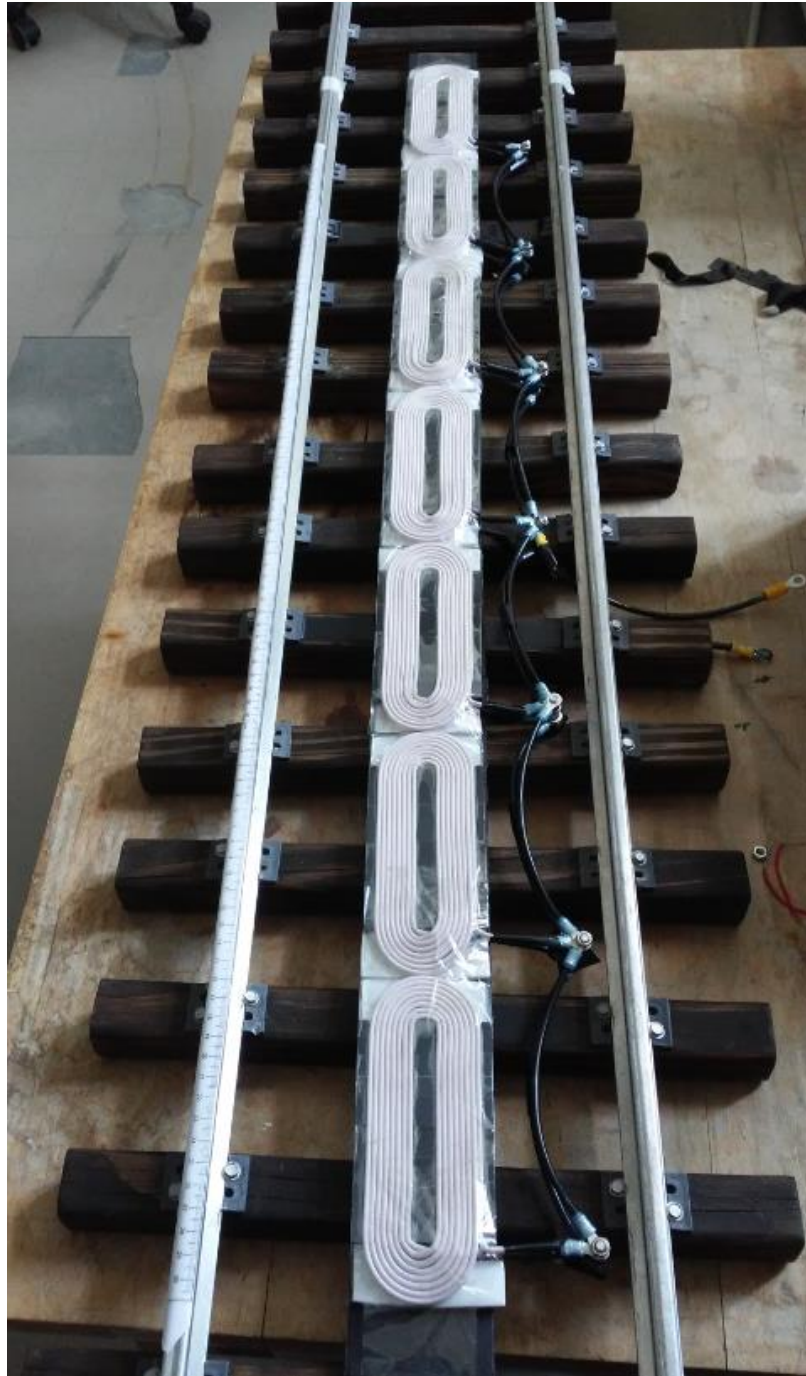
Figure 4-16 E-core Coils Transmitters
