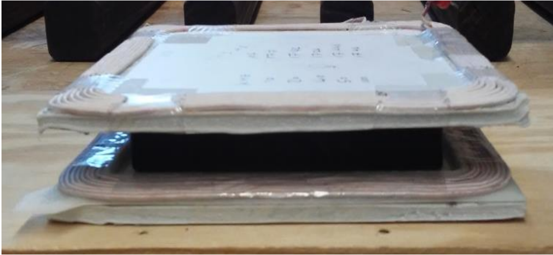
Figure 3-2 One-to-One Air Coils with a Core
