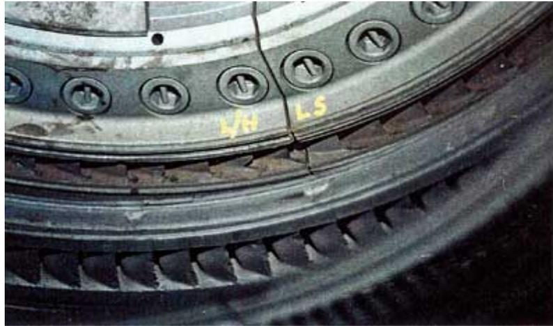
Figure 3.12: Nozzle Block Solid Particle Erosion (*Courtesy: TG Advisers Inc.*) [52, 53]
