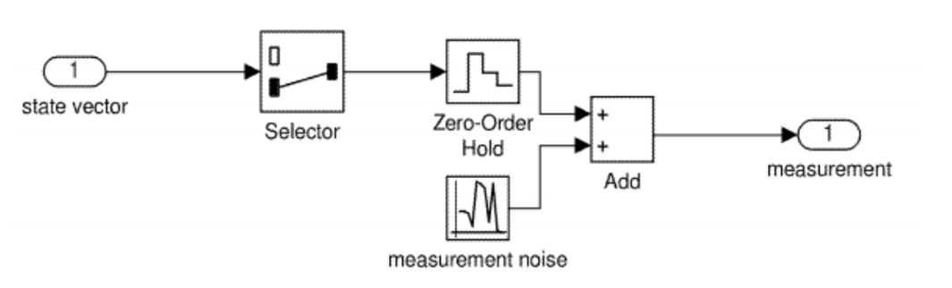
Figure 5.1: Model of the time discrete noisy sensor in Simulink
