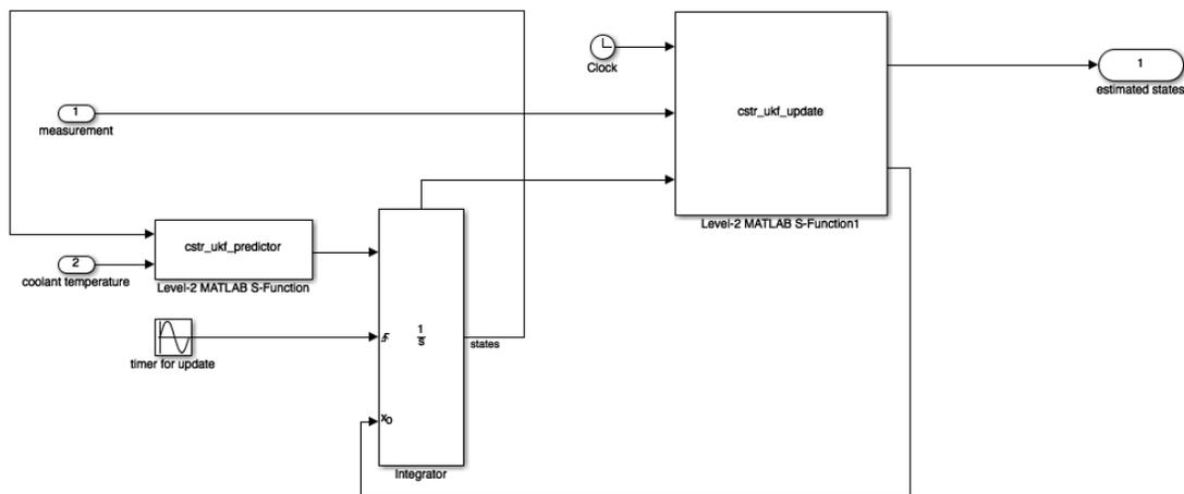
Figure 5.2: Model of the Unscented Kalman Filter
