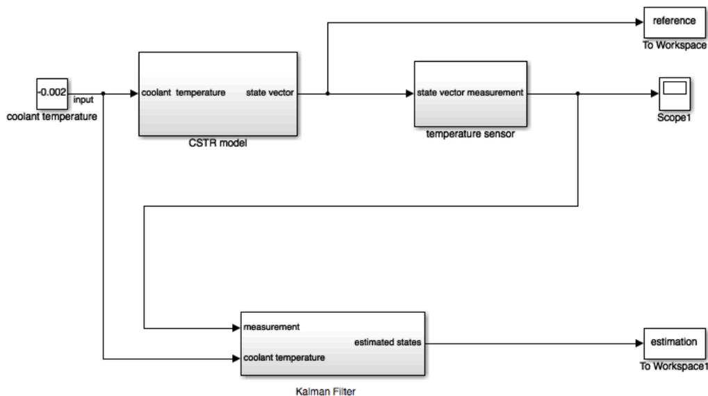
Figure 5.3: Complete Implementation of Kalman Filter in Simulink(KF)
