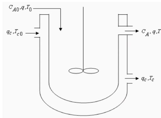
Figure 4.1: Schematic diagram of a Continuous Stirred Tank Reactor
