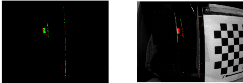
Figure 4.15: Events generated by movement of speaker driver
