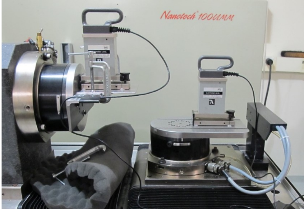
Figure 5.21: Electronic levels setup for measuring roll in the X carriage and pitch in the Z carriage before the environmentally controlled enclosure was installed.
