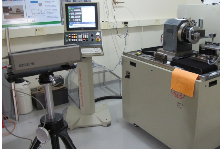
Figure 5.36: Laser interferometer setup for measuring the linear displacement error in the X carriage.
