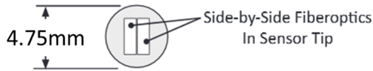
Figure 5.47: Philtec fiber optic probe configuration showing the sensor tip [5].
