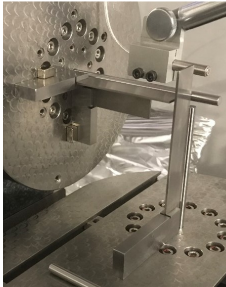
Figure 5.1: Using precision ground shafts and machinist squares to align the rotational axes of the B and C carriages and to align the capacitance gage with the fiducial origin.
