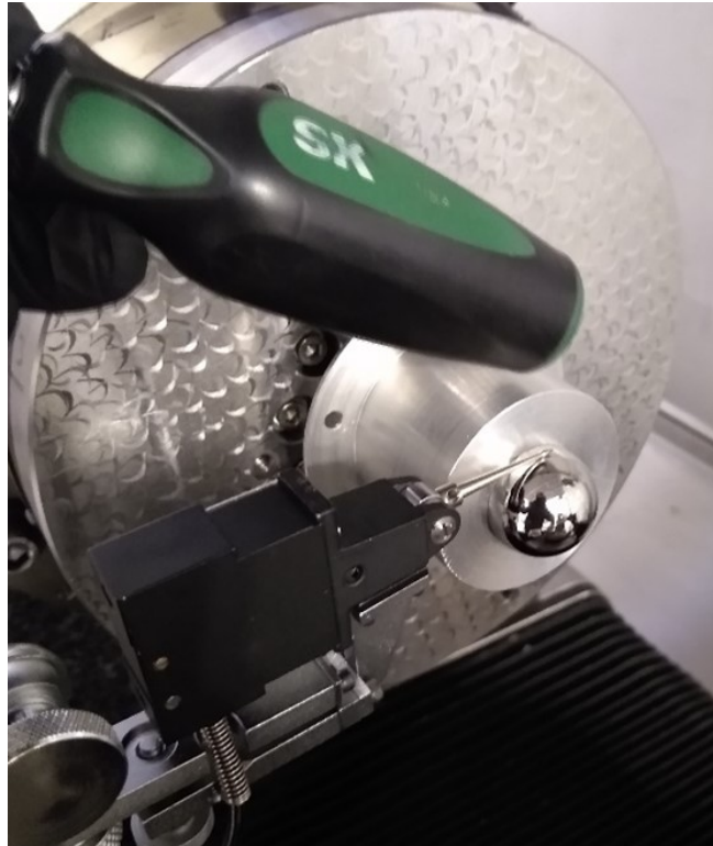
Figure 4.3: Centering the 1-inch steel ball using an electronic indicator and rubber handled screwdriver for centering the probe on the rotational axis of the C carriage.
