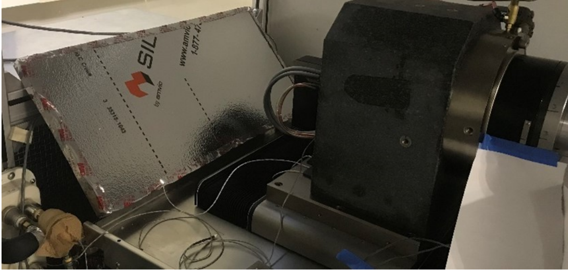
Figure 2.11: Directing the downdraft from the plenum over the machine rather than into the return ducting.
