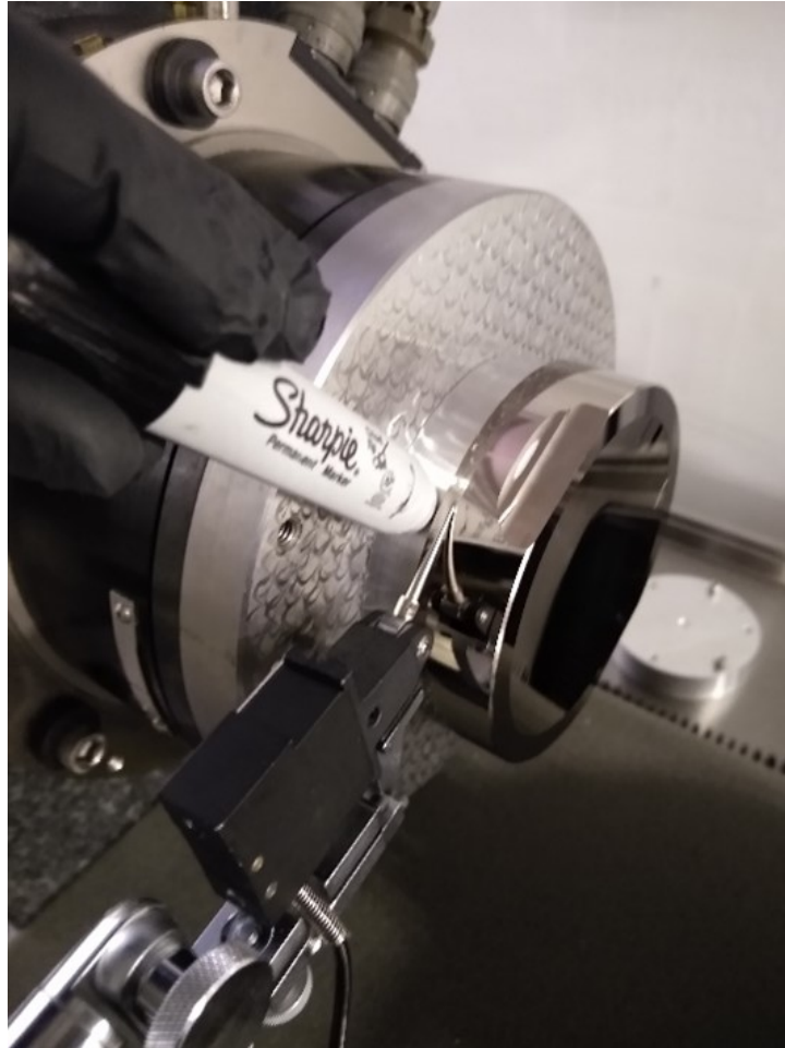
Figure 7.8: Centering the part using a permanent marker to keep from damaging the diamond turned outer diameter.
