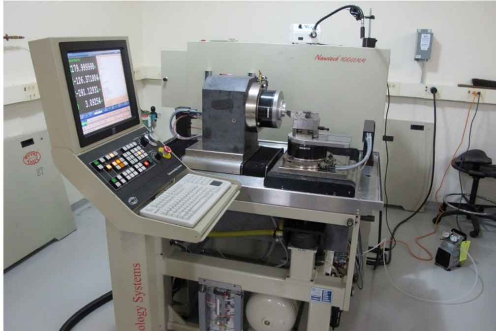
Figure 2.1: Moore Nanotech 100UMM before the environmentally controlled enclosure was installed.
