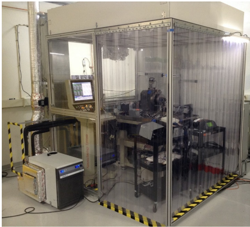
Figure 2.5: Moore Nanotech 100UMM surrounded by the environmentally controlled enclosure showing the chiller, curtains and plenum.
