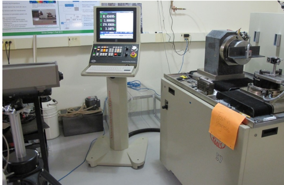
Figure 5.34: Optical setup for the linear displacement measurement of the Z carriage including the laser.
