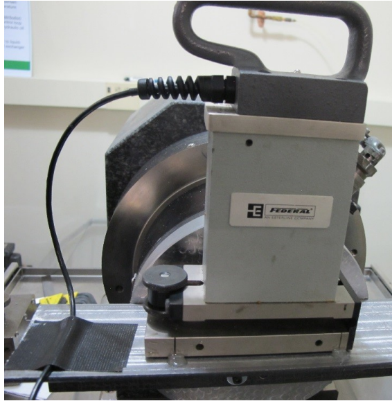
Figure 5.16: Attaching the electronic level using 5 min. epoxy and tape to secure the wire.
