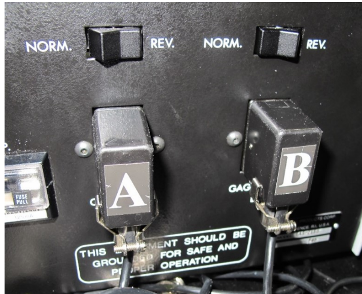
Figure 5.15: Switching the sign of the signal from the electronic levels using the switches on the back of the signal analyzer.
