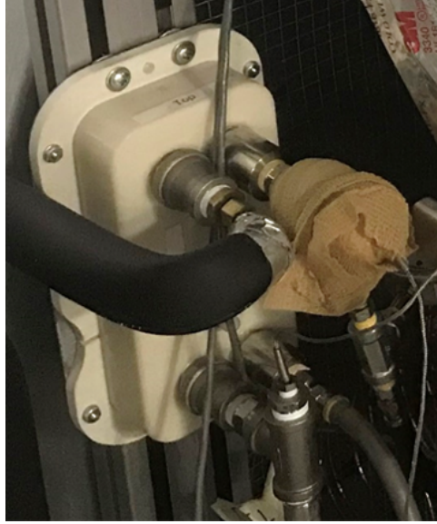
Figure 2.7: Heat exchanger for the hydraulic oil using the chiller water and resistive heater to control the oil temperature.
