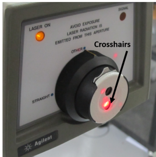
Figure 5.31: Agilent laser system alignment using the crosshairs to align the optics to return the laser to the inlet.
