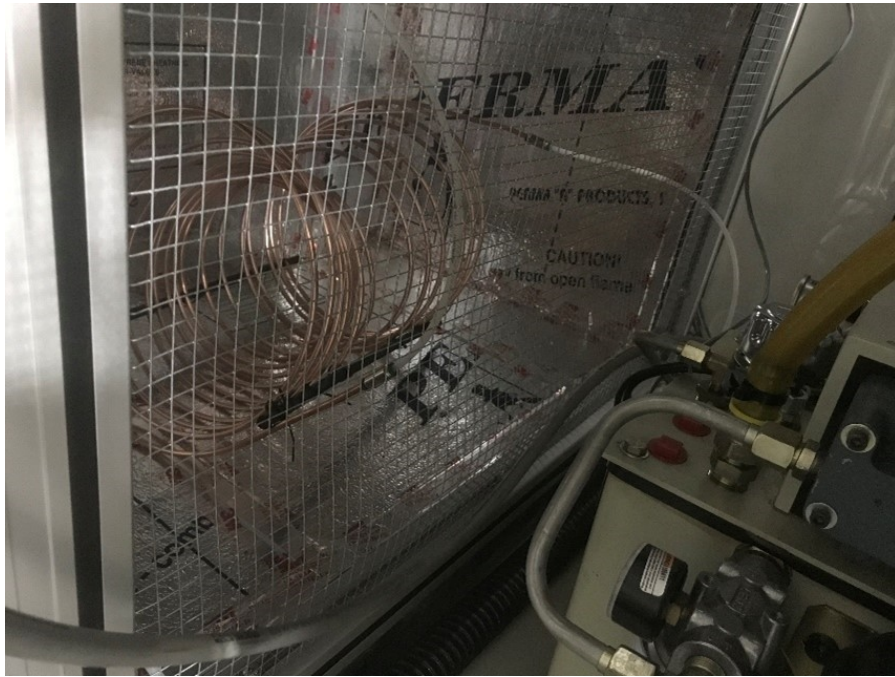
Figure 2.10: High pressure air heat exchanger made from copper tubing in the air return ducting for the environmentally controlled enclosure.
