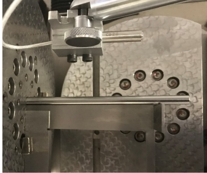
Figure 5.2: Showing the top view of the alignment process for the rotational axes of the B and C carriages.
