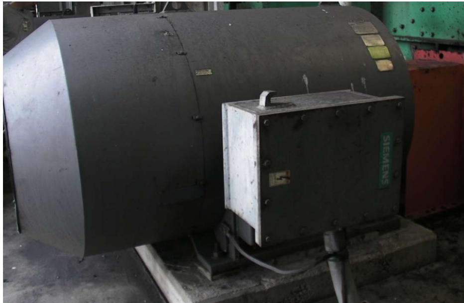
Figure 3.5: Picture of 600 HP coal crusher's induction motor.
