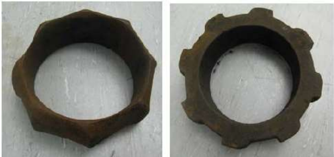
Figure 3.7: Coal crusher hammers: Picture on the left shows the degraded hammer removed from the coal crusher and picture on the right shows the replacement of the degraded hammer.
