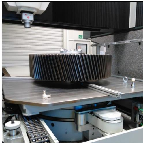
Figure 1.11. WES gear loaded on a hydrostatic rotary table at the Bremen Institute for Metrology, Automation and Quality Science (BIMAQ), University of Bremen, Germany.
