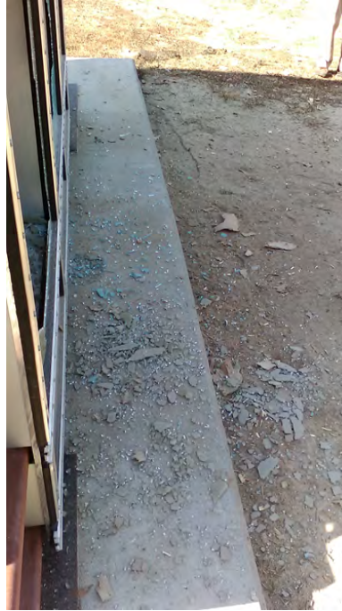
FIGURE 4.19: Exterior debris generated by failure of Lite 4 in suction during Test 6
