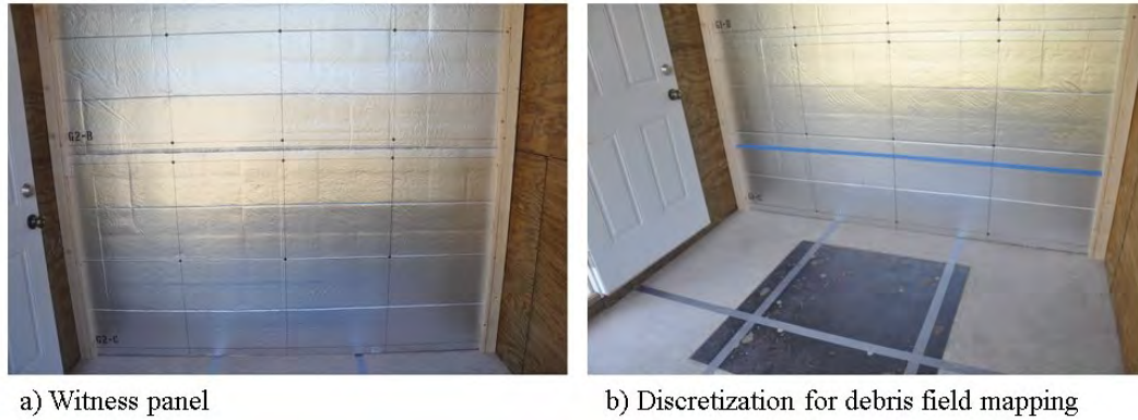
FIGURE 4.6: Witness panel and discretization of the enclosure floor for debris field mapping
