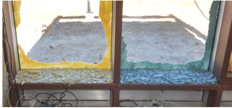
FIGURE 7.10: Photograph of debris that landed on the facade framework during Test 5
