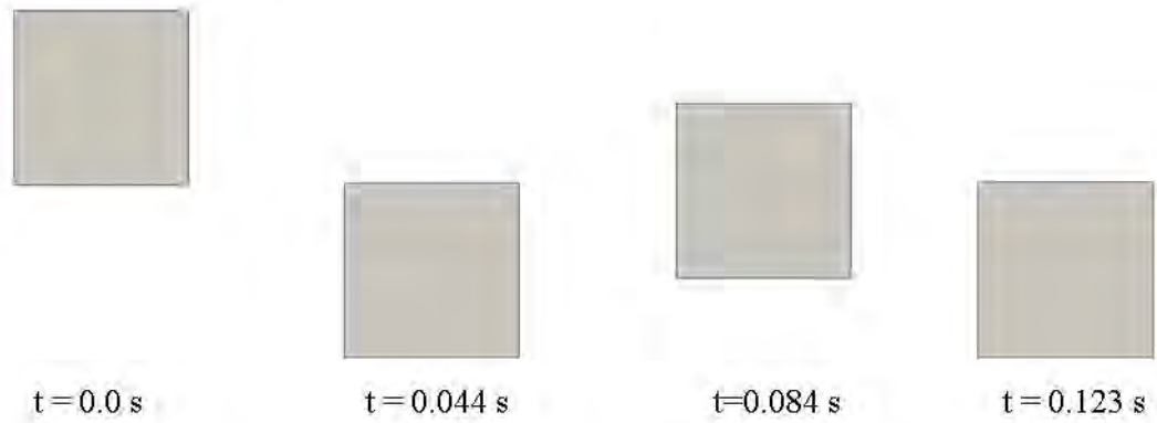
FIGURE 3.28: Paraview rendering of a single AEM element falling under gravity and rebounding with a coefficient of restitution of 0.9
