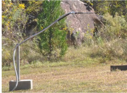
FIGURE 4.11: Typical installation of a free-air pencil probe to capture incident overpressures
