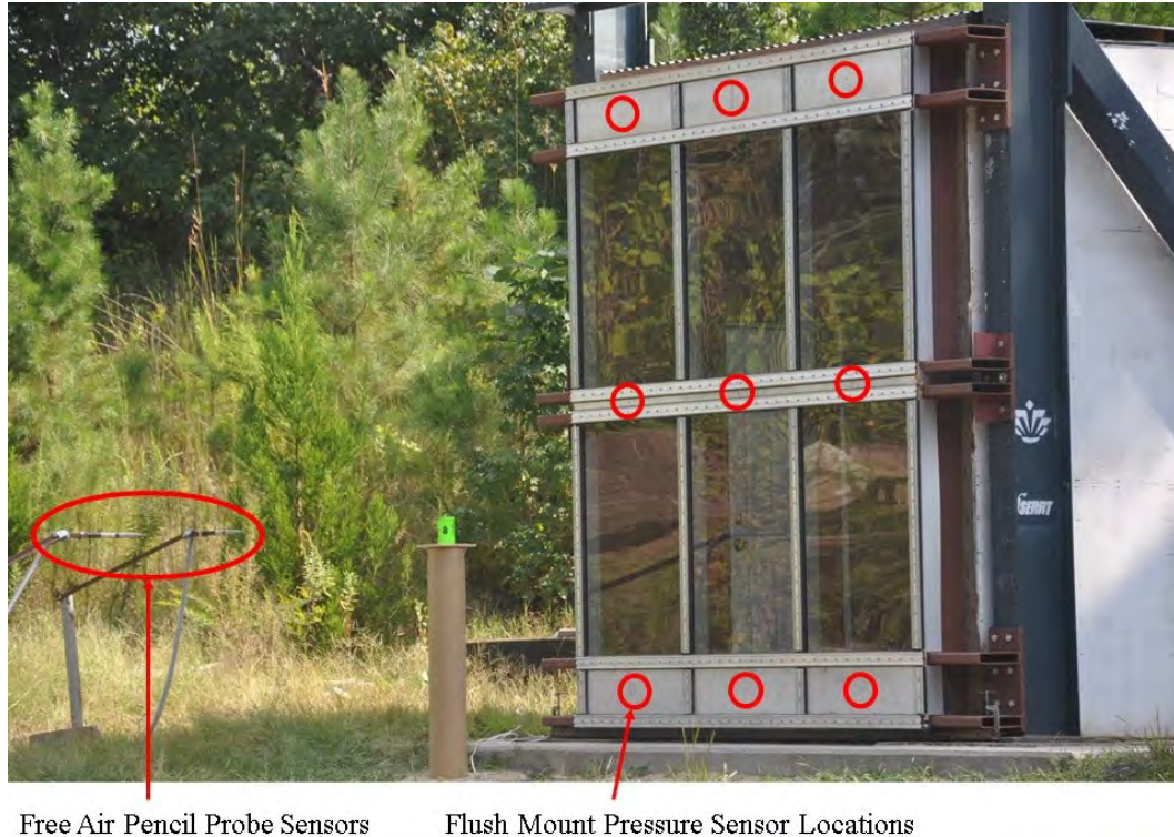
FIGURE 4.12: Photograph of typical array of blast overpressure transducers
