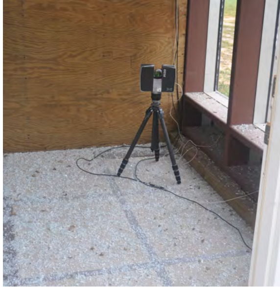
FIGURE 4.8: Deployment of the LiDAR scanning system to the interior debris field
