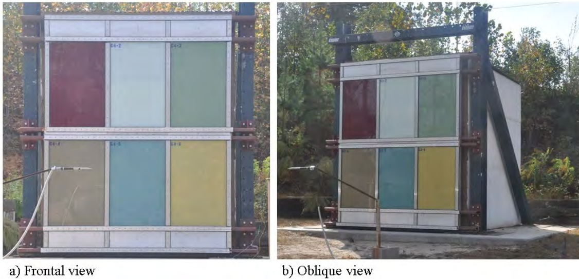
FIGURE 4.1: Photographs of the test structure featuring a facade front outfitted with glass lite specimens
