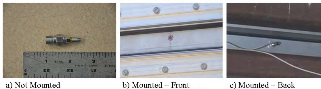
FIGURE 4.9: Typical installation of a flush mount pressure sensor in the facade
