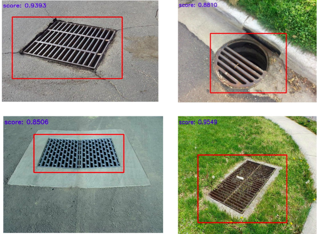
Figure 5.3: Qualitative results showing the basic localization on random unseen images with variety of drop inlet
