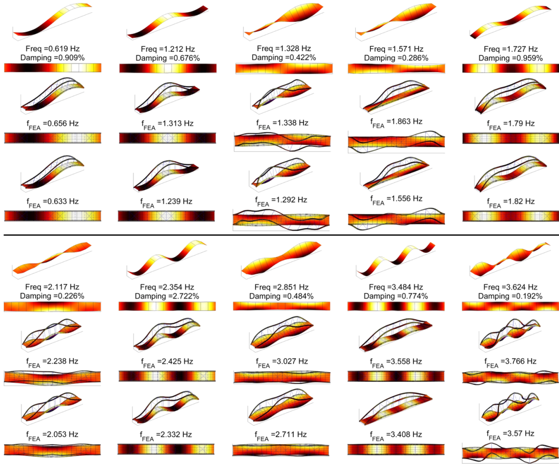
Figure 23: Modal parameter estimates associated with modes one through ten extracted from the experimental measurements (row#1), idealized model (row#2), and calibrated model (row#3)
