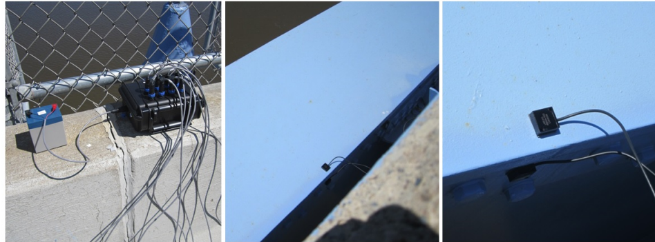
Figure 6: Wireless sensor network powered by an external battery (left). Proximity of accelerometer to the top inner edge of the tie girders (middle). Accelerometers oriented to measure vertical and lateral accelerations (right).
