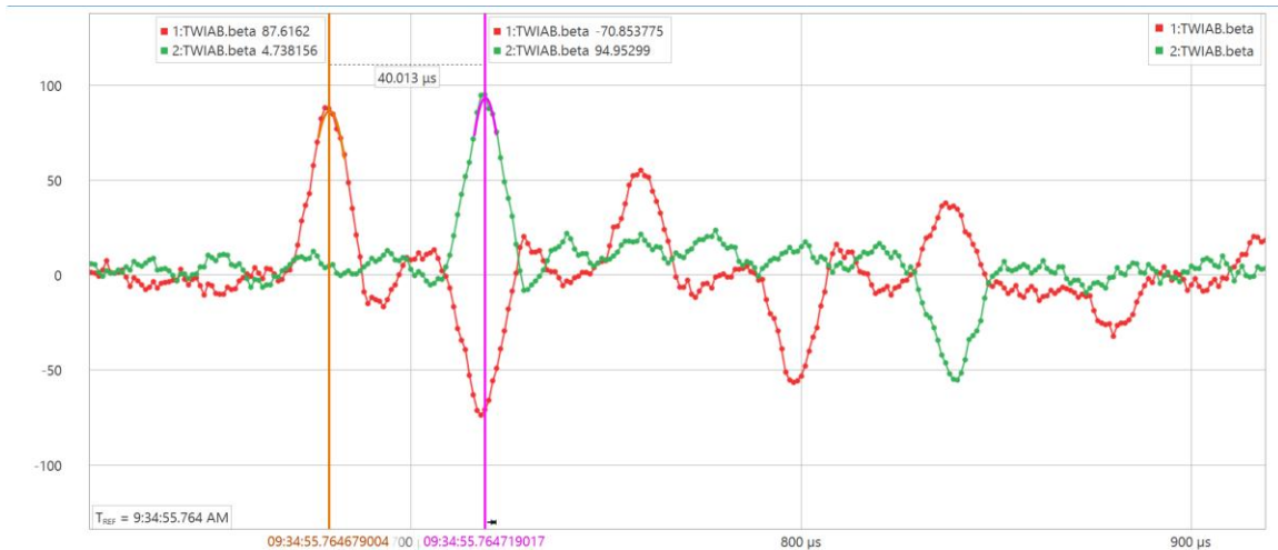
Figure 5.14 TW Beta Currents for AB Fault at Middle-of-the-Waveform
