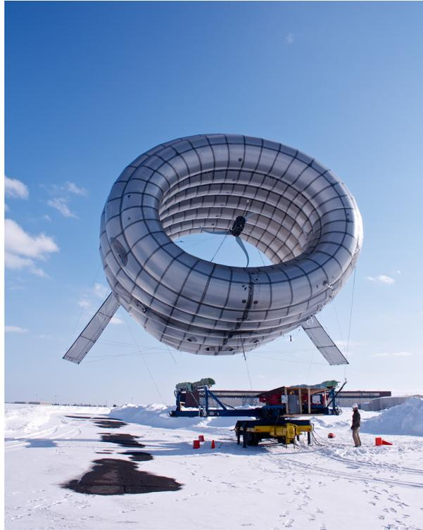
Figure 3: Full-scale prototype of Buoyant Airborne Turbine (BAT) during 2012 flight testing at Loring Air Force Base. [31]
