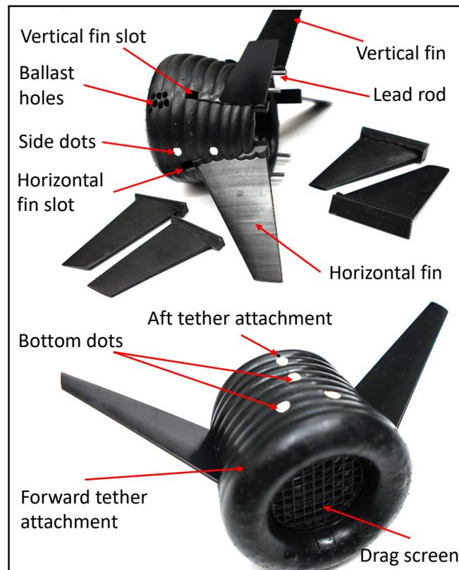
Figure 7: Image of 3D printed scaled model of BAT illustrating the rapid reconfigurable features.
