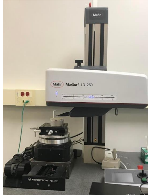
FIGURE 45: Mahr Profilometer LD 260 measuring a DT surface located in the Metrology Suite
