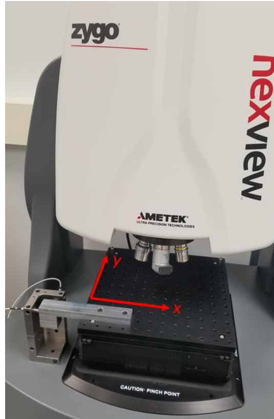
FIGURE 39: Second part of setup of capacitance probe testing with NexView stage, Al bar extension, capacitive sensors and their housing
