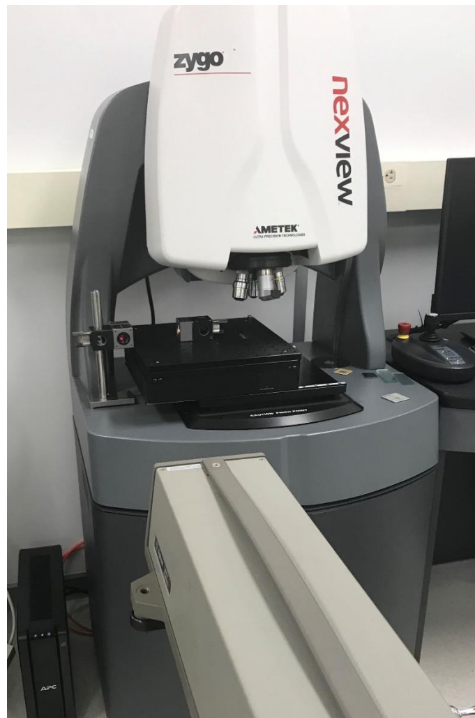
FIGURE 34: DMI set up on the NexView stage
