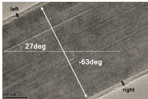
FIGURE C.3: The illustration of diameter measurement.
