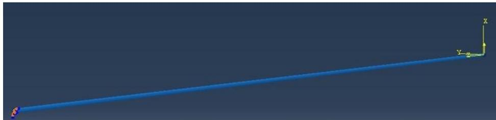
FIGURE D.7: The solid wire with a boundary condition and a concentrated force.
