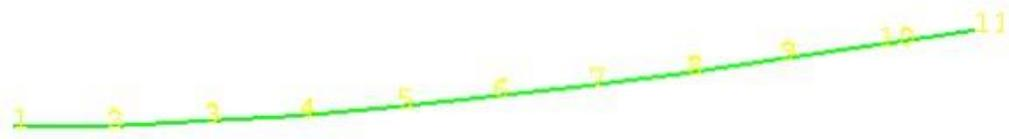
FIGURE D.2: Result of a beam bending under this load (10 elements).
