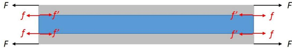
FIGURE 4.18: Schematics of tensile test on a NW (blue) with an oxide layer (grey).
