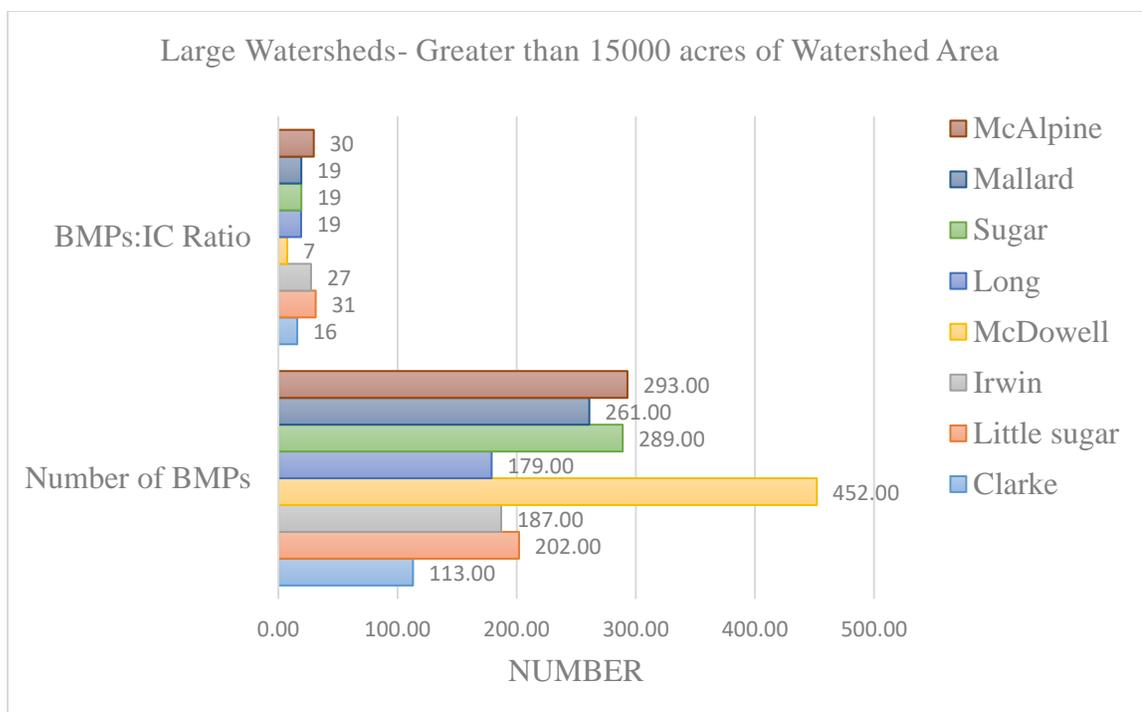
**Figure 21: Comparison of BMPs and BMPs IC ratio in large watersheds**
