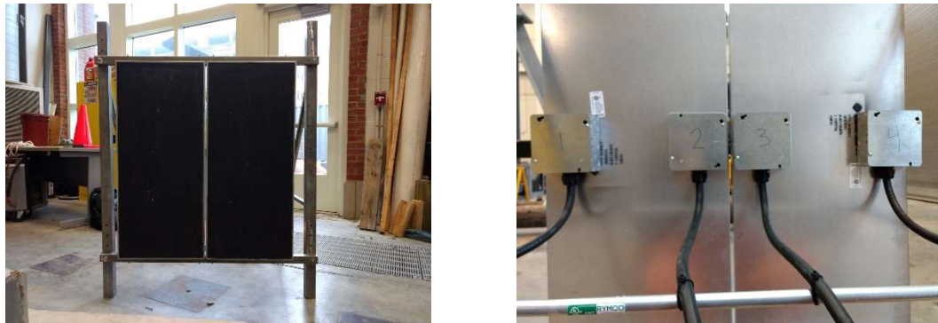
FIGURE 4.14: (a) Front view of testing frame. (b) Rear view of panels with protective connection plates.
