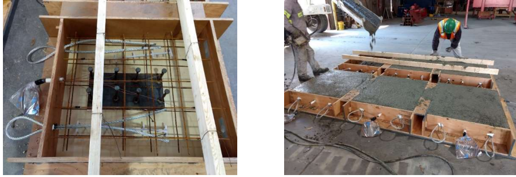
FIGURE 4.10: (a) Top down view. (b) Pouring and vibration of specimens.
