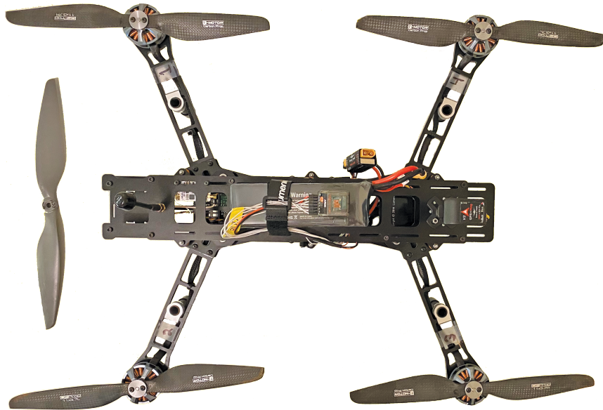
Figure 4.1: Picture of drone used in Experiment 1. Drone equipped with 11x3.7 propellers in picture; 12x4.5 propeller shown on left for reference.
