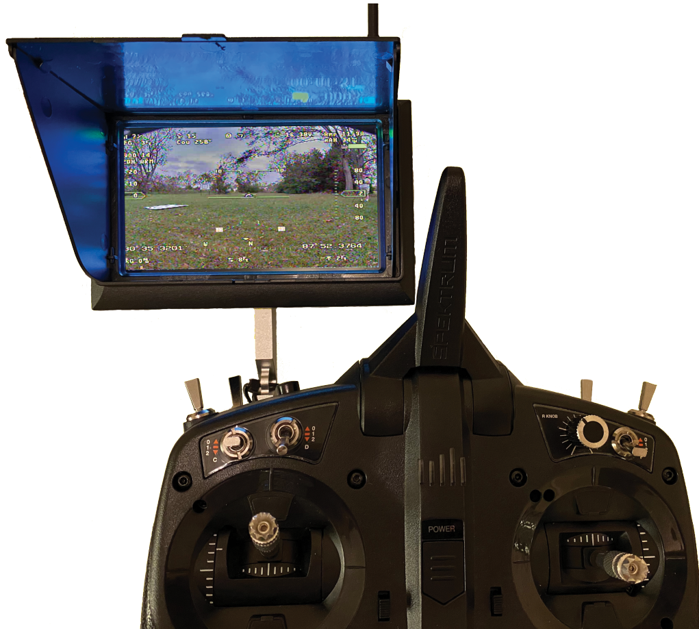
Figure 4.2: Picture of RF transmitter with a standard 4.3 inch LCD monitor used in Experiment 1.
