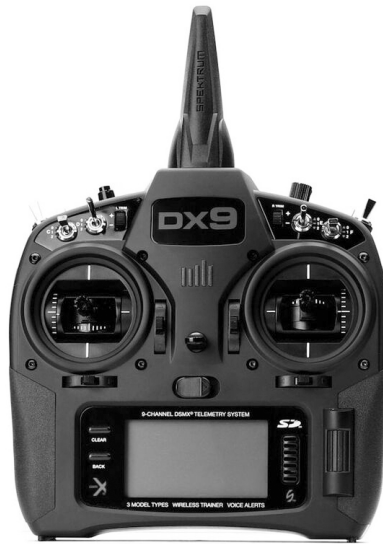
Figure 2.4: Typical RF transmitter used for remote-control aircraft operation. Image courtesy of Horizon Hobby, LLC.
