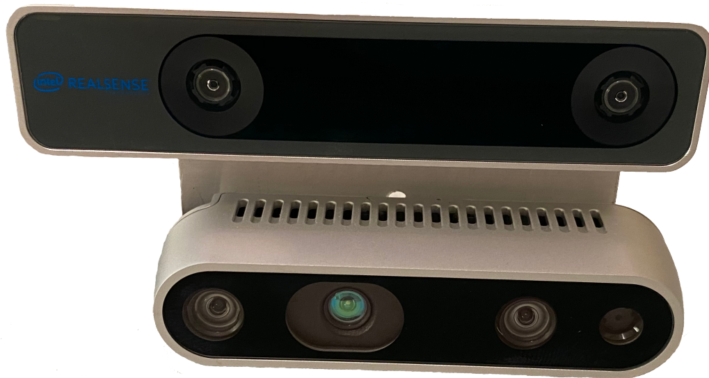
Figure 3.9: Image of Intel RealSense T265 tracking camera module mounted with D435 depth camera.
