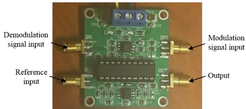
Figure 5-10- Compact lock-in amplifier circuit using AD630 microchip [87].
