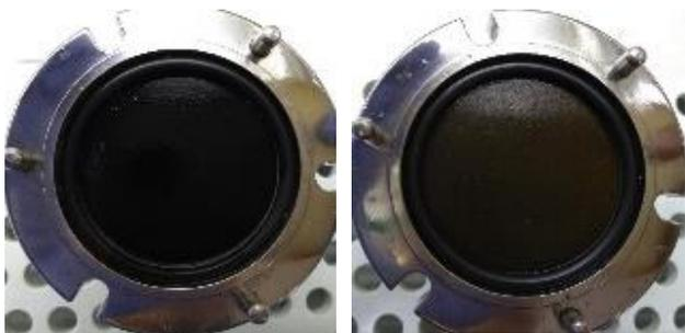
Figure 3.2: NanoResin membrane before any breakthrough experiments (left) and then after the 3<sup>rd</sup> breakthrough experiment (right). Yellow tinge on thin film (right) is from the NaFL adsorption.
