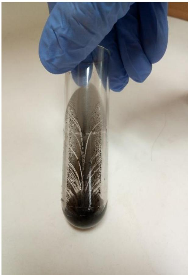
Figure S2.1: After centrifugation at 100,000 RCF (1 h), the reaction mixture deposits at the wall of the polycarbonate tubes
