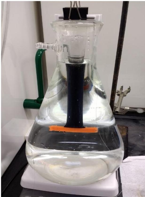
Figure S2.2: Brine removal from Aq-SNR dispersion. (A) Aq-SNR is added in the form of dialyte and MilliQ is added as dialysate. The dialysate was replaced after every 2 h and then conductivity of dialysate was checked as a function of the number of iterations. This confirms maximal removal of brine ( $<1 \mu\text{S}/\text{cm}$ ).
