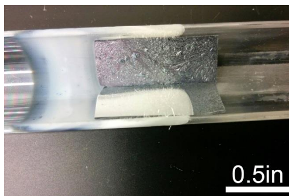
Figure 2-25. Repeating the side-by-side experiment, the target substrate, without the catalytic droplet, was positioned next to the catalytic substrate which has 30 \mu\text{l} 1M NaOH at the temperature range of 280-585°C.
