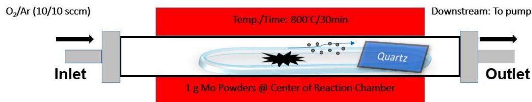
Figure 3-5. Schematic set up of residue production experiment on quartz substrate
