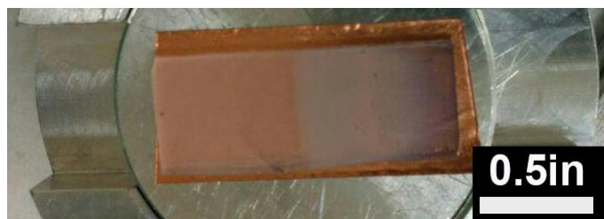
Figure 3-3. Schematic of glass substrate after growth on SEM plate (copper tape underneath); white deposition on right side (low temperature area), no deposition on left side (high temperature area).
