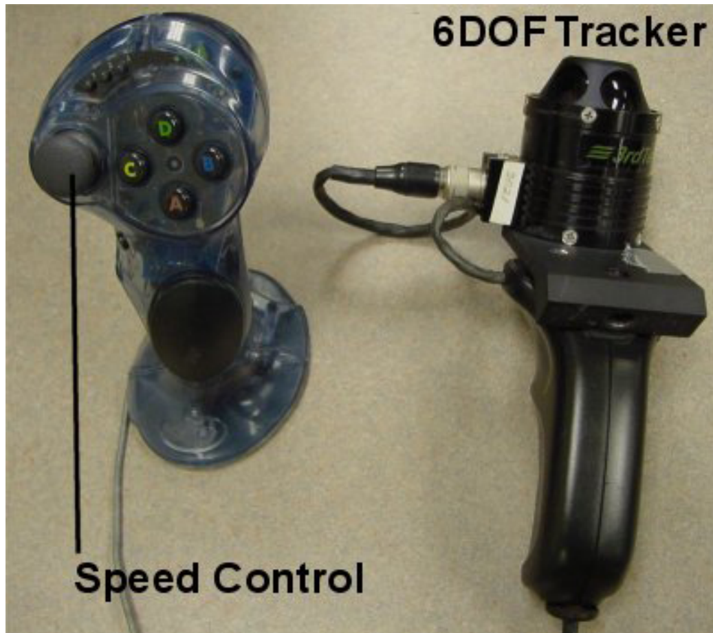
Figure 3.2: The devices used for virtual travel in Experiment 1. Movement was triggered using a button on the tracked device held in the dominant hand. Velocity was controlled using the thumbstick held in the non-dominant hand.
