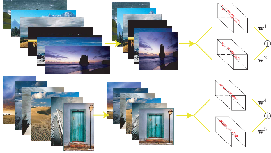
Figure 3.6: Grouping strategy to reduce computational overhead: The integer dilated Convs can be shared by properly grouped images according to aspect ratios.
