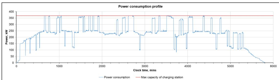
FIGURE 54: Power consumption profile for arrival rate of 12 veh/hour with BAR and charging station's design with non-sharable pumps only.
