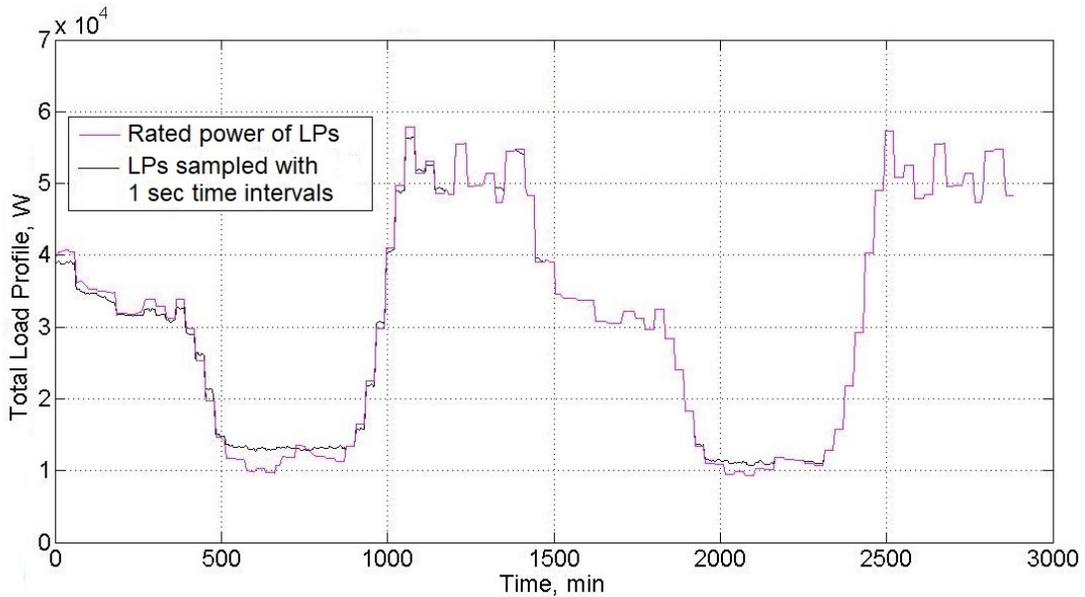
FIGURE 25: Total load profiles (TLPs) calculated for two scenarios: rated power of LPs and LPs sampled with 1 sec time intervals.
