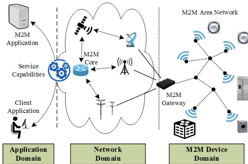
FIGURE 13: Main domains of the M2M reference architecture according to European Telecommunications Standards Institute.
