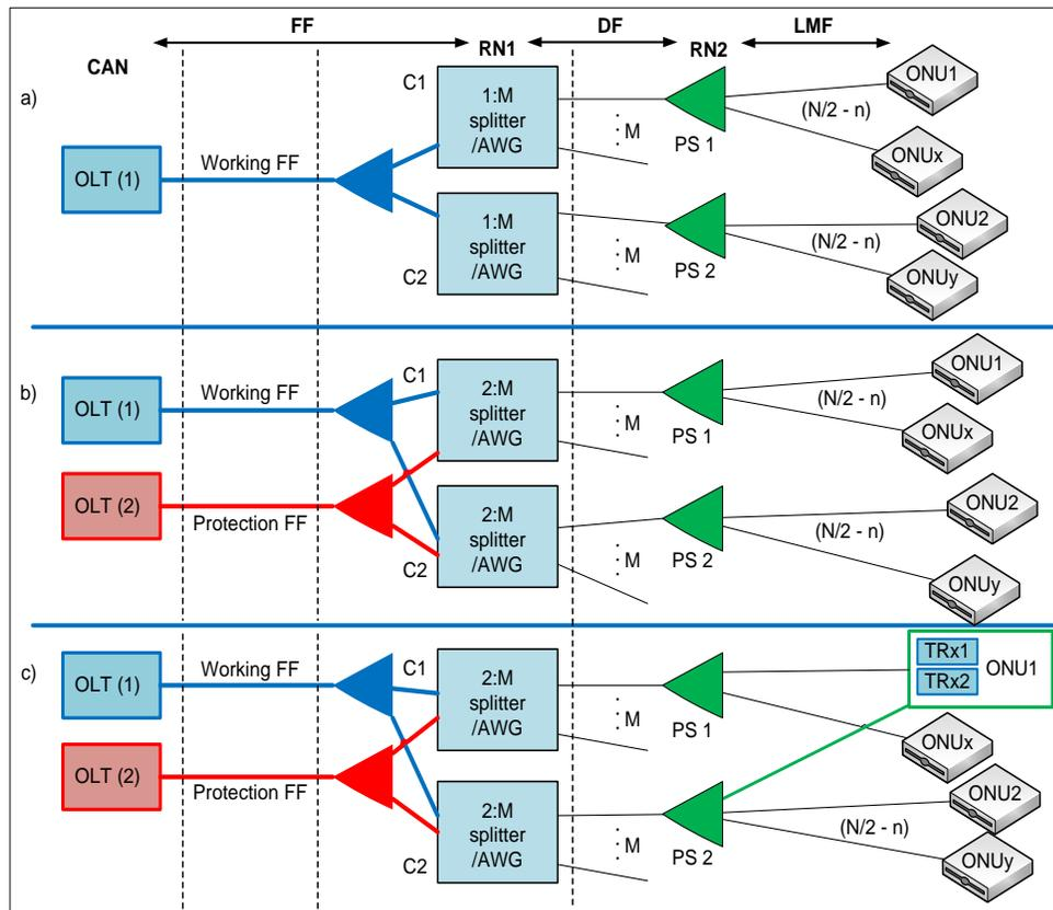
FIGURE 20: PON architecture: (a) without protection; (b) with protection up to RN1 for all connected ONUs; (c) E-to-E protection for some selected ONUs [153].
