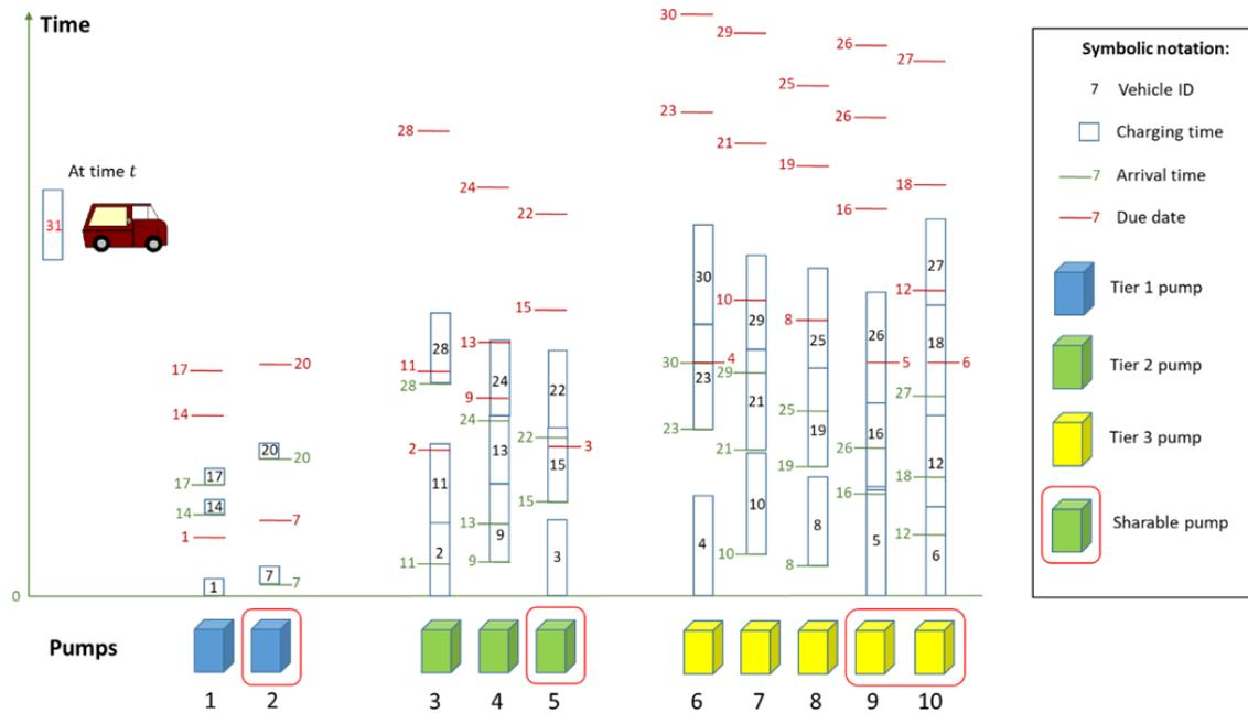
FIGURE 30: An example of optimal scheduling procedure scenario represented as a snapshot at the time of new vehicle arrival. Sharable pumps in each tier are framed in red.
