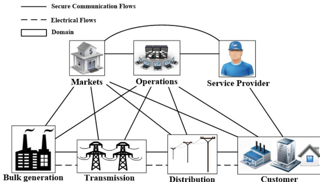
FIGURE 2: NIST Smart Grid Conceptual Model.
