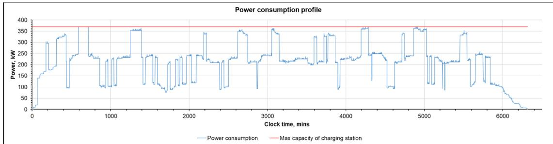
FIGURE 53: Power consumption profile for arrival rate of 10 veh/hour with BAR and charging station's design with non-sharable pumps only.
