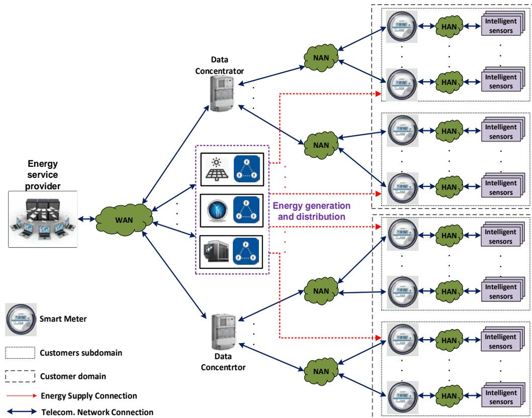
FIGURE 12: General example of telecommunication network supporting advanced metering infrastructure of SGs. Data from each customer domain is obtained through corresponding data concentrators and NANs, which consist from several HANs that are monitored by smart meters. WAN controls energy generation and distribution for the whole grid.
