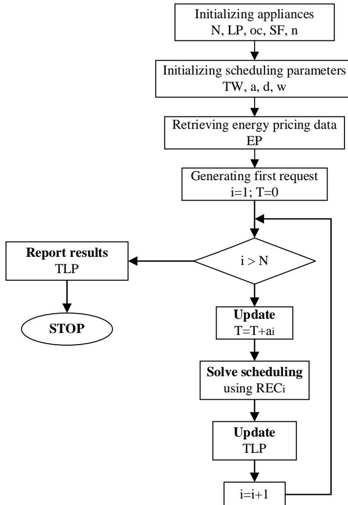
FIGURE 22: Flow chart of simulation implementation for dynamic load scheduling.
