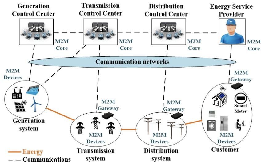
FIGURE 16: Mapping of the proposed M2M communications architecture onto the European Telecommunications Standards Institute (ETSI) M2M architecture applied to the Smart Grid.
