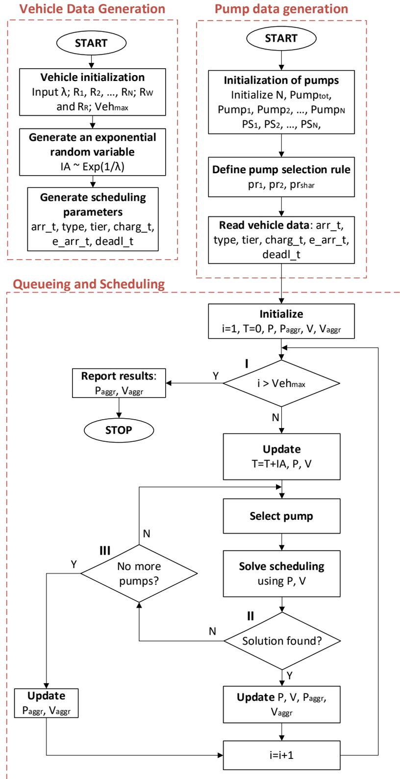
FIGURE 31: Flow chart of a simulation implementation of the online scheduling procedure
