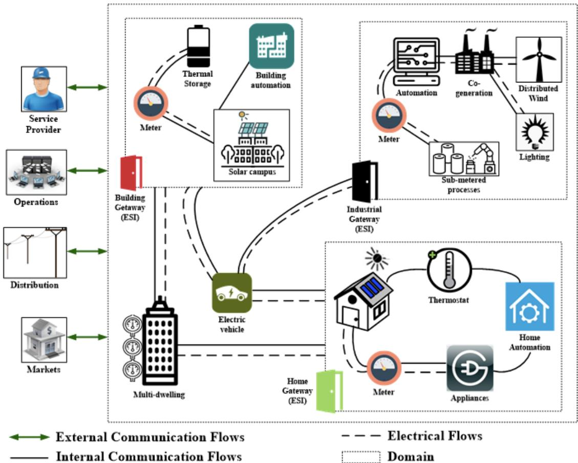
FIGURE 3: General architecture of the customer domain.
