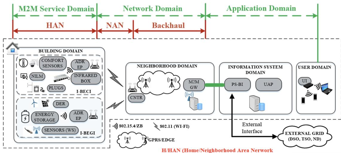
FIGURE 15: Overall system architecture, highlighting the relation with the standardization work.
