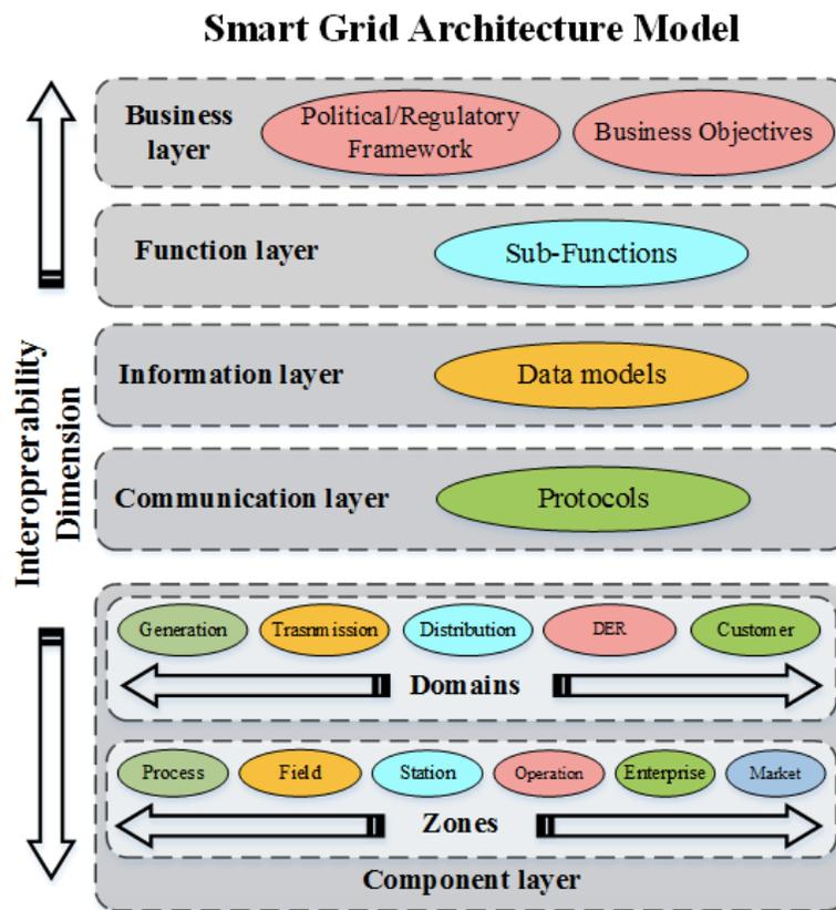
FIGURE 11: Smart Grid architecture model. The component layer refers to the domains of the SG conceptual model (see FIGURE 2).
