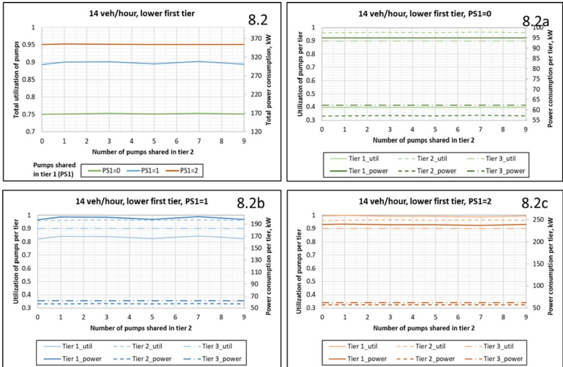
FIGURE 48: Utilization of pumps for 14 veh/hour arrival rate with lower first tier vehicle ratio vs number of pumps shared in tiers 1 (PS1) and 2.
