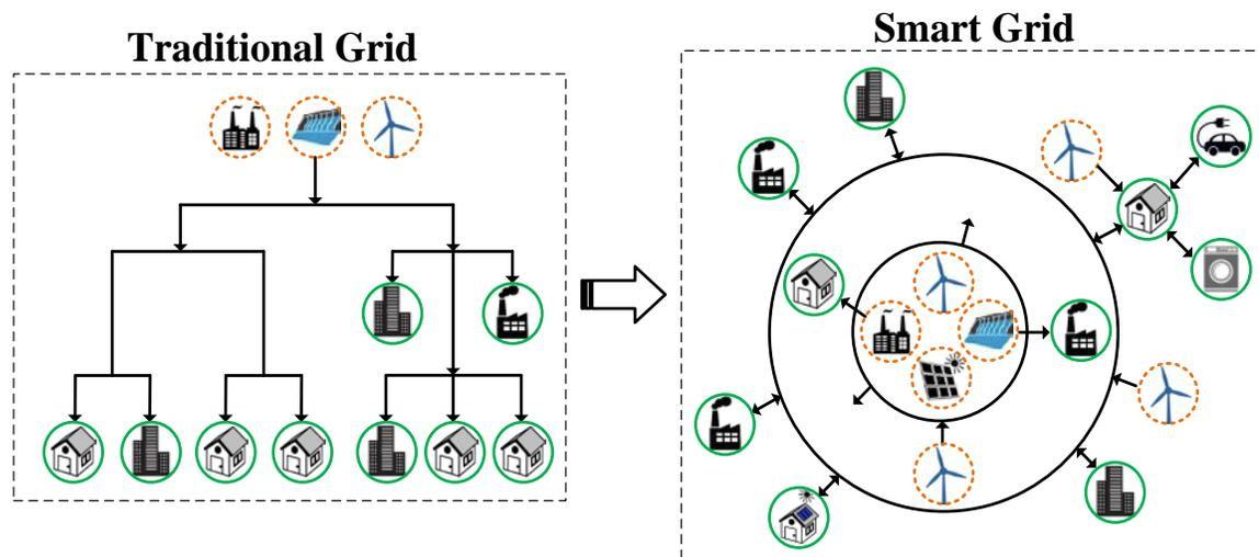
FIGURE 1: Transition from traditional grids to smart grids.
