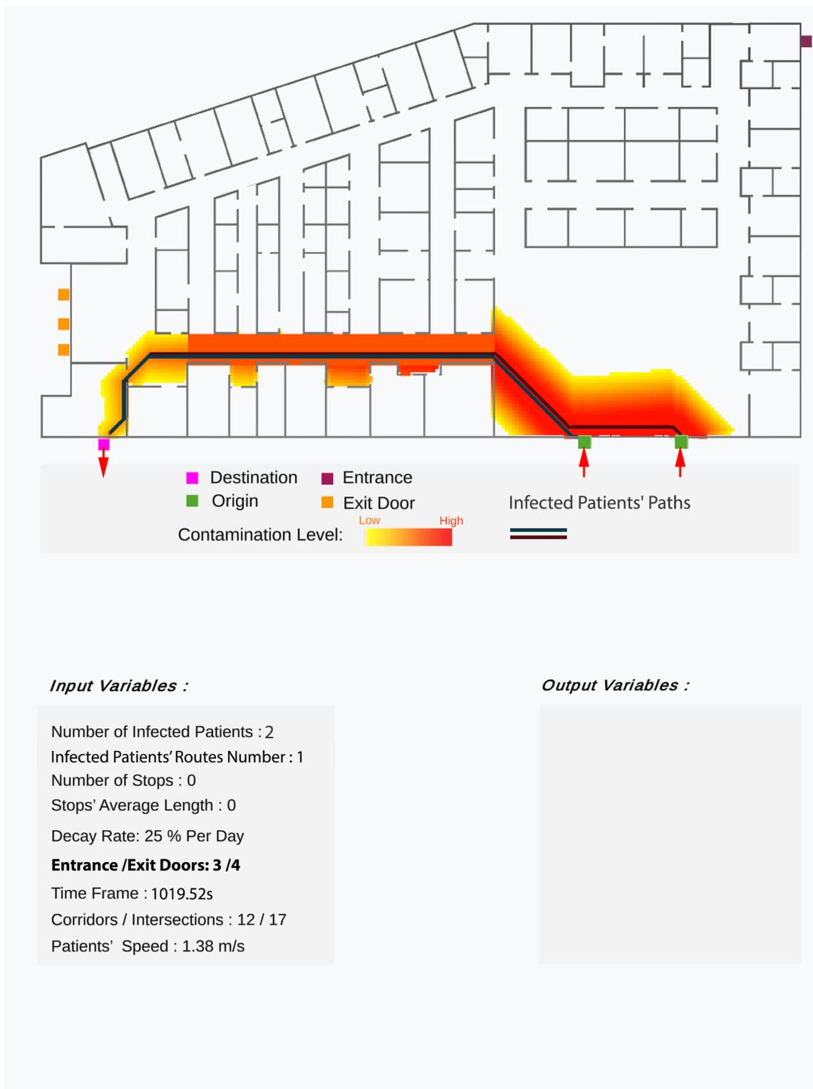
Figure 4.21: The simulation of virus spread by two infected patients to investigate the effect of the location of entrance and exit doors on the infection probability in a hospital
