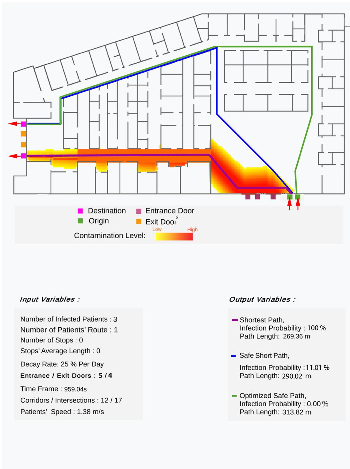
Figure 4.28: The illustration of the generated shortest, safe short, and optimized safe paths and their lengths and infection probabilities
