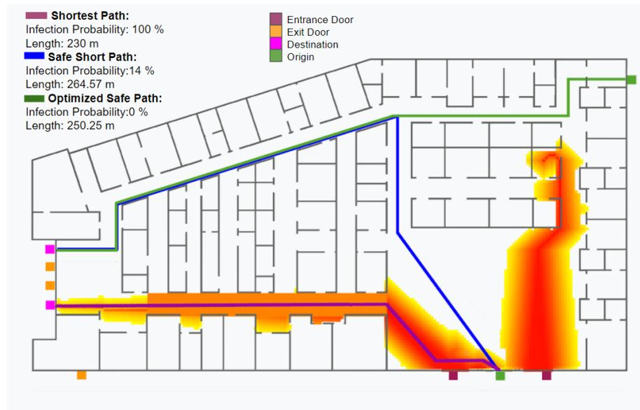
Figure 3.15: The Shortest, Safe Short & Optimized Safe Routs' Infection Probabilities
