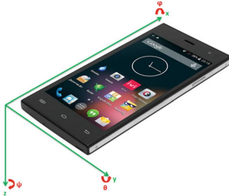
Figure A.35: The coordinate system of smartphones and corresponding orientation angles
