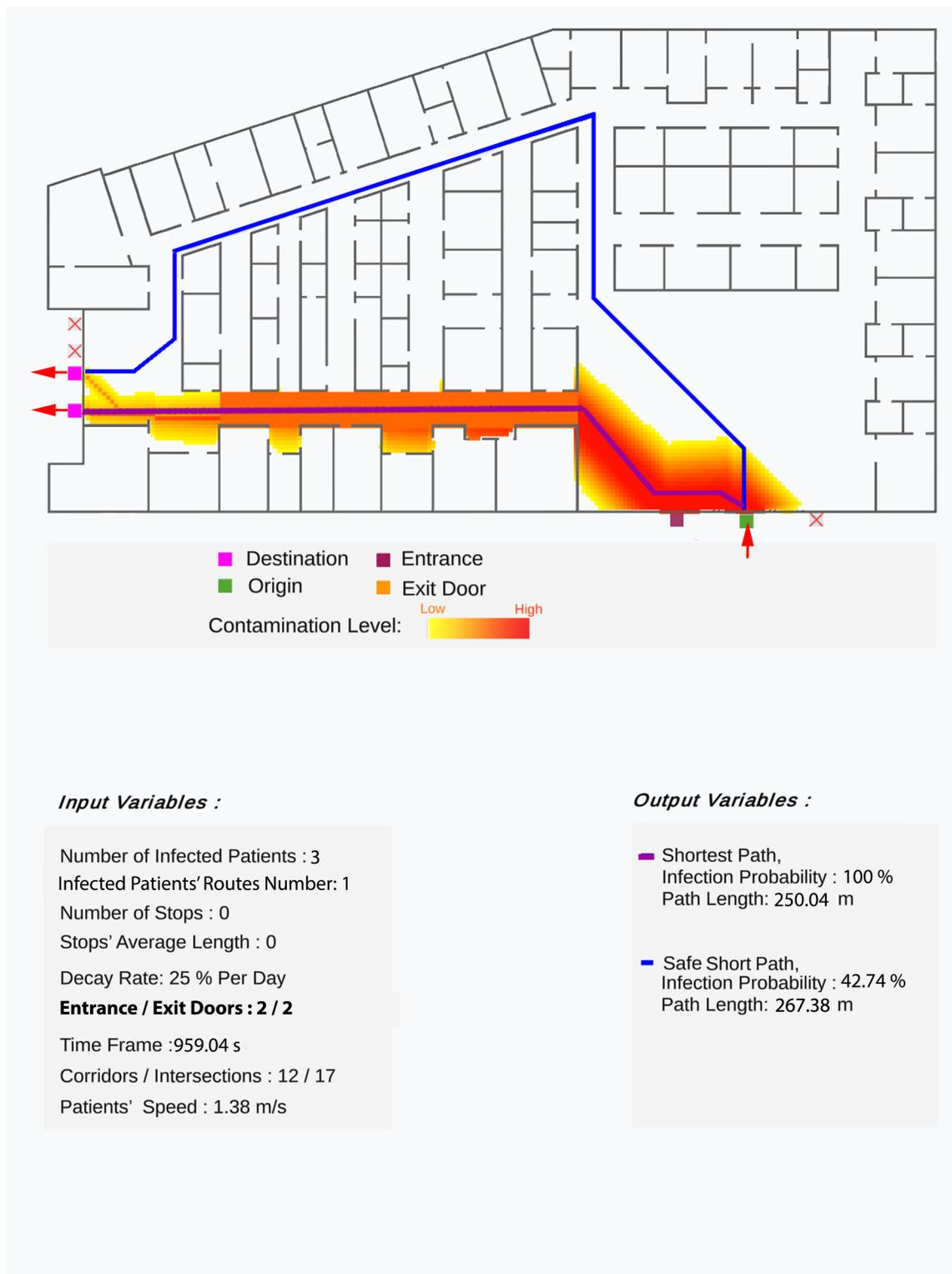
Figure 4.24: The illustration of the generated shortest and safe short paths and their lengths and infection probabilities
