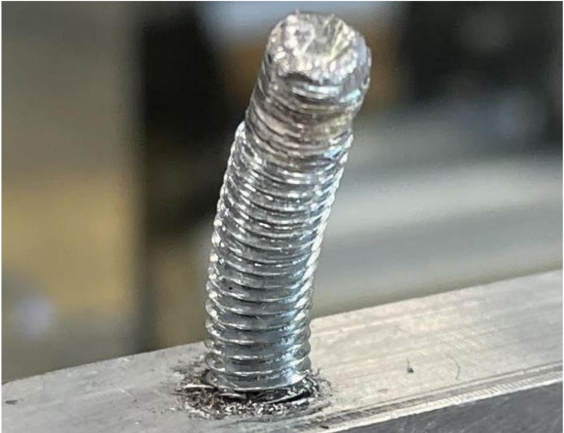
Figure 6.9: Four of the M5 wing nuts stripped out the threads and were pulled off the M5 studs.
