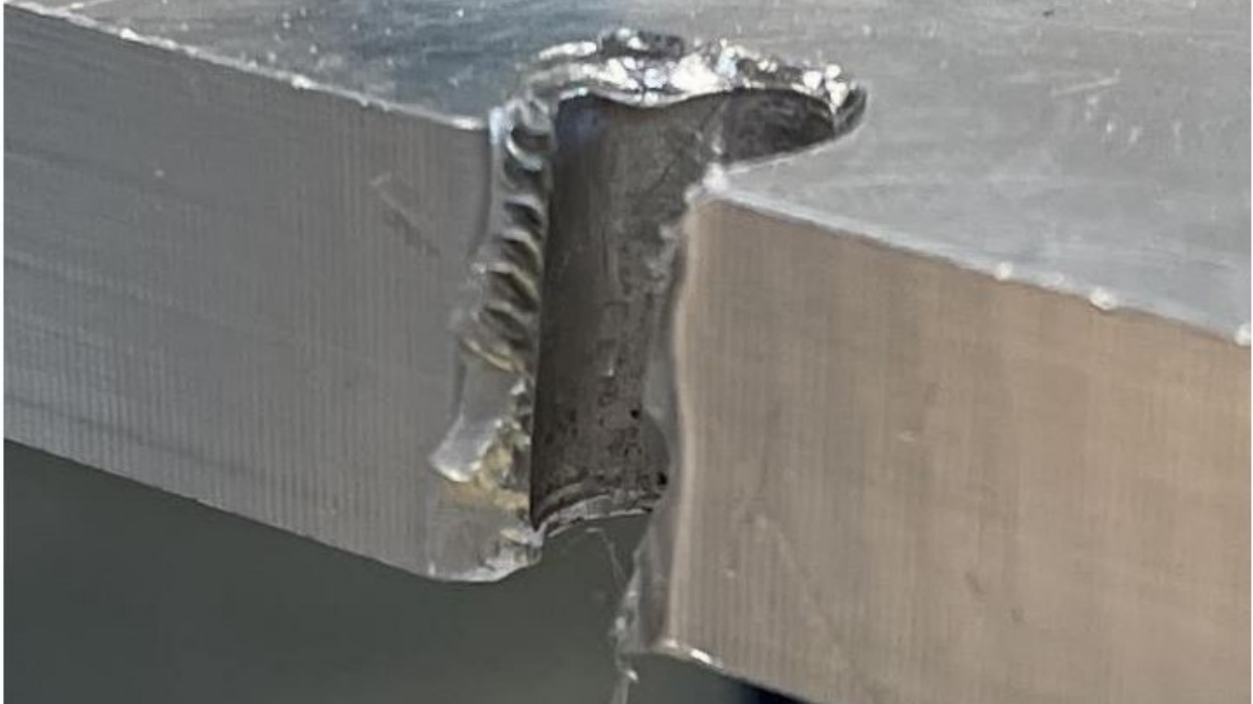
Figure 6.10: The last of seven studs was intake but the aluminum lid pulled laterally through it and cut a slot.
