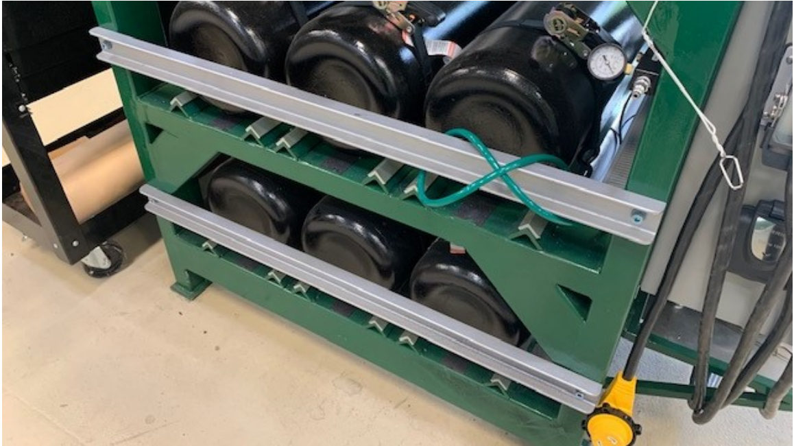
Figure 3.8: Image of the UNCC HSWT frame retention C-channel safety bars.
