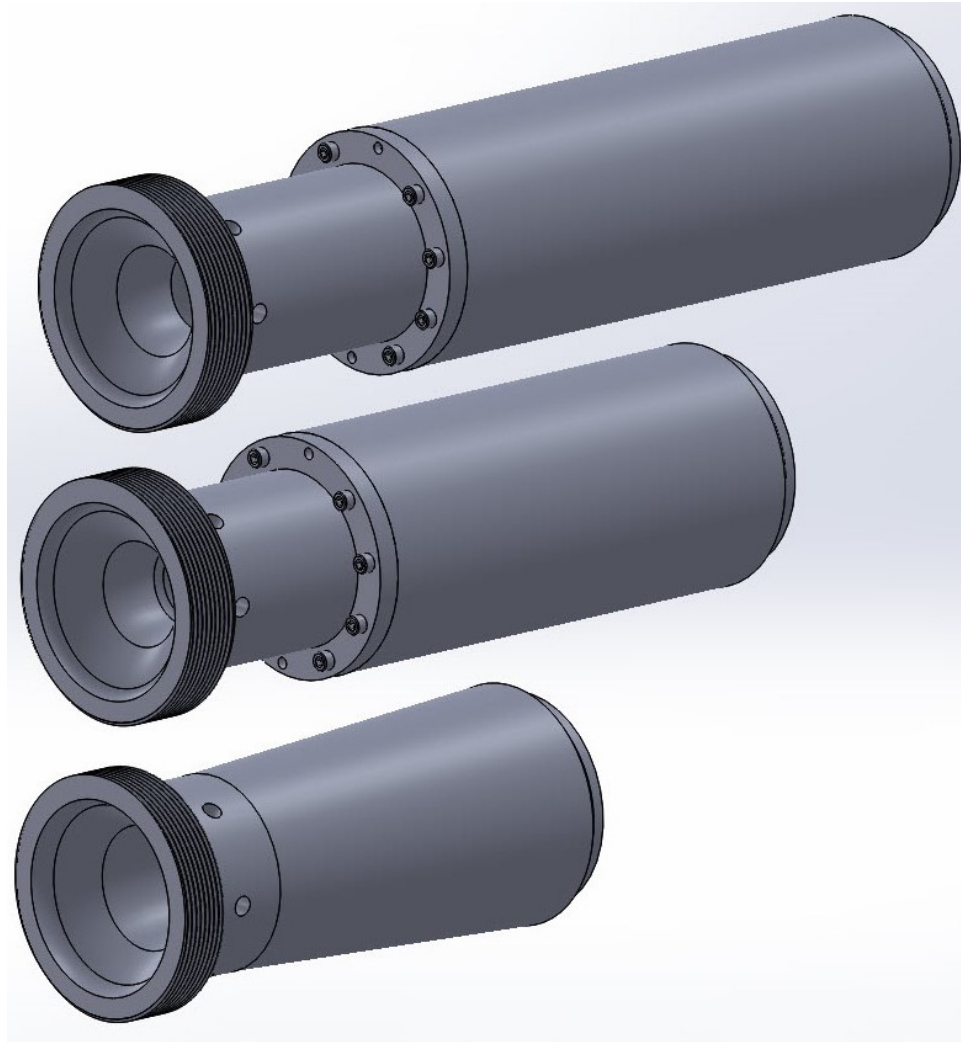
Figure 3.22: CAD image of the Mach 3, 5, and 7 CD nozzles.
