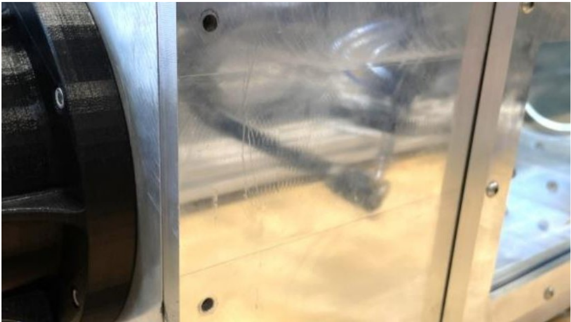
Figure 6.12: Two of the side M5 fasteners popped completely out of the chamber.
