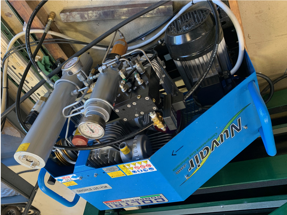
Figure 3.13: Image of UNCC HSWT Nuair air compressor.
