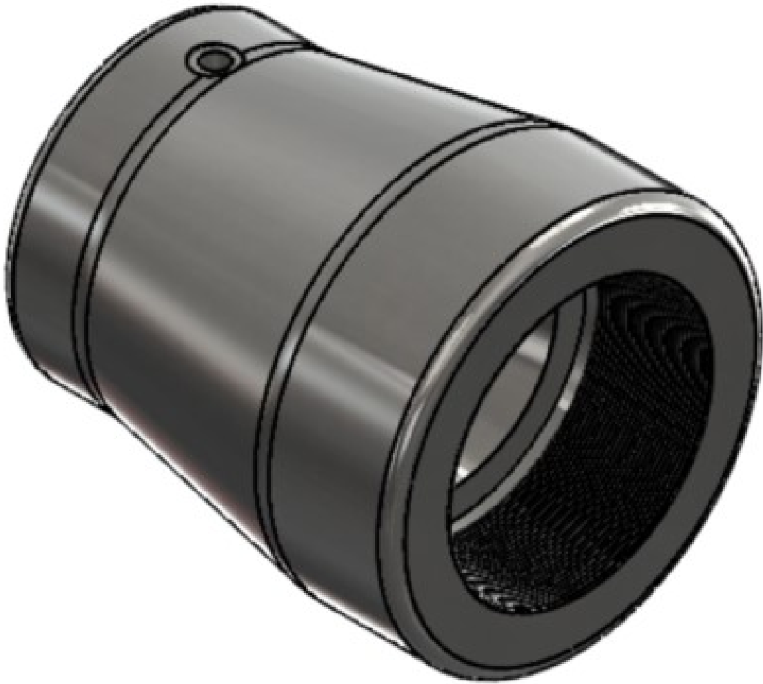
Figure 3.19: CAD image of the benchmark hypersonic tunnel plenum.
