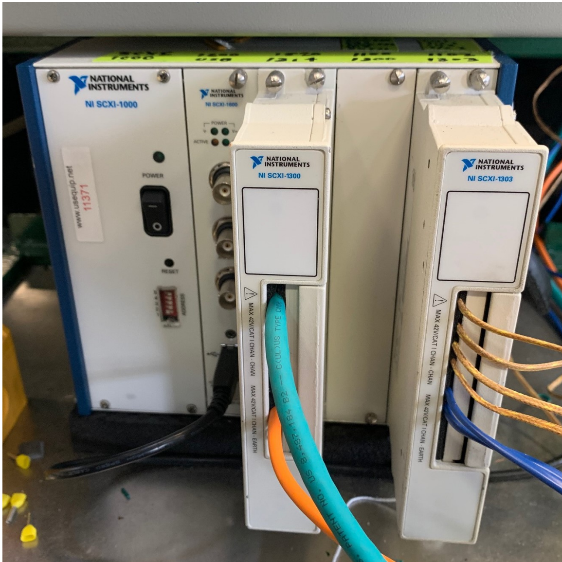
Figure 4.11: Image of the National Instruments SCXI 1000.
