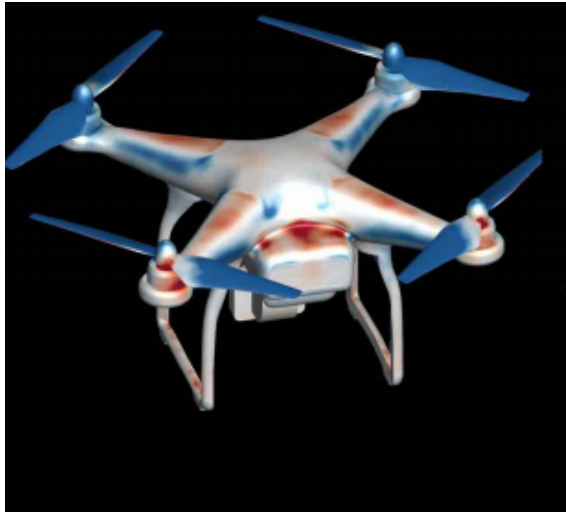
Figure 2.9: Surface pressure coefficient of DJI phantom 3 when viewed from above[12].
