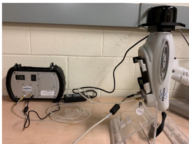
Figure 4.6 PHXRF connected to a vacuum pump
