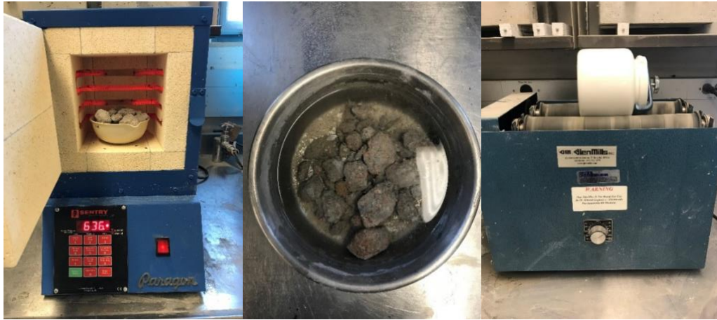
Figure 3.6 Thermal shock method test apparatus (from Mamirov et al. 2020)
