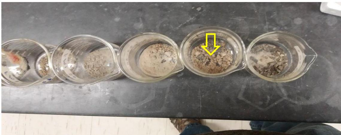
(Figure 1.1). Subsamples from core FM1. A fine layer of silt was found preserved between the sharp contact of the sand lens and marsh facies in the younger storm layer. The yellow arrow indicates the sample containing the silt layer.
