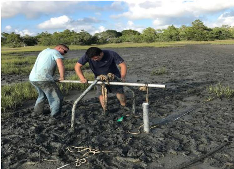
(Figure 4.1-B) Lance Zurawski and Steven Ortiz using the pry-and-lever system to remove a vibracore.
