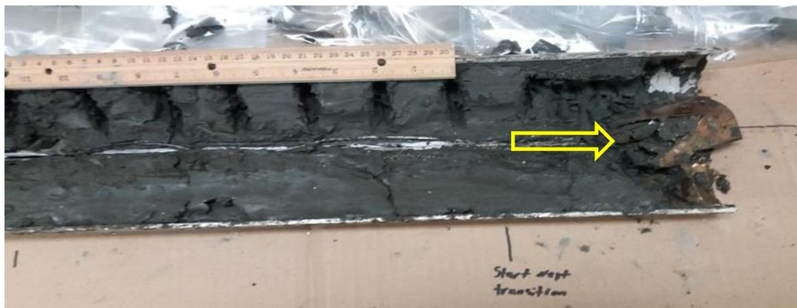
(Figure 4.2) Remnant of sediment catcher applied to prevent sample loss at yellow arrow.
