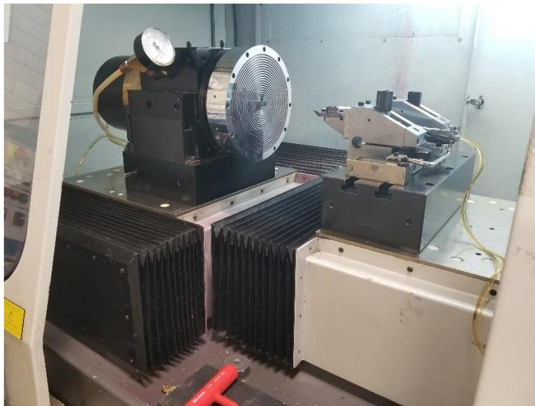
Figure 4.10 Precitech 350 diamond turning machine
