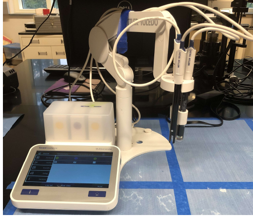
Figure 4-7. The Mettler Toledo probe used to measure the EC and pH of the saturated CCR extract.
