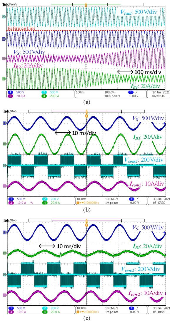
**FIGURE 19.** Voltage regulation waveforms. (a) Branch currents and voltage waveforms of the source and load. (b) Converter 2 waveforms when injecting positive voltage. (c) Converter 2 waveforms when injecting negative voltage.
