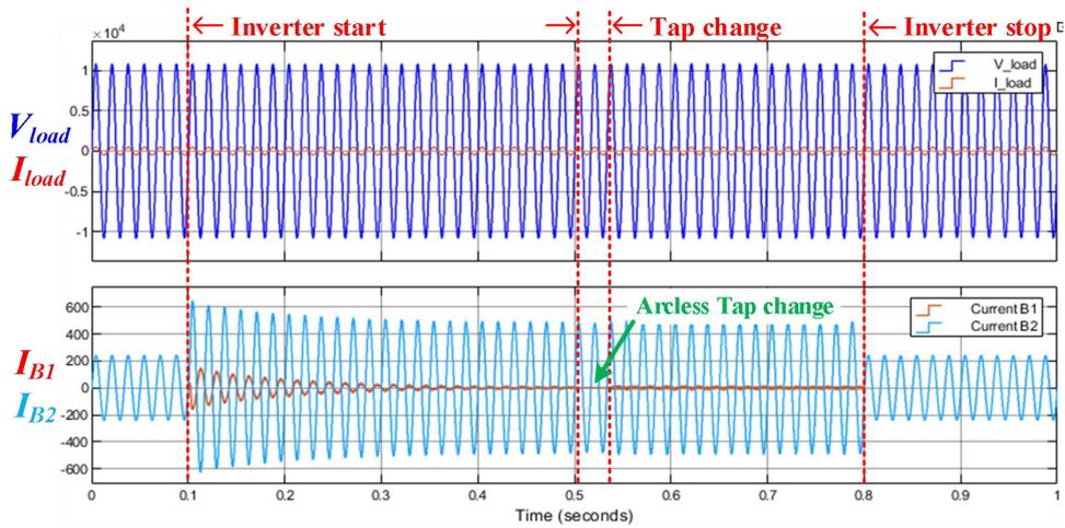
**FIGURE 10.** Arcless tap change mode simulation results.
