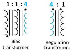
**FIGURE 6. Transformer turns ratio.**
