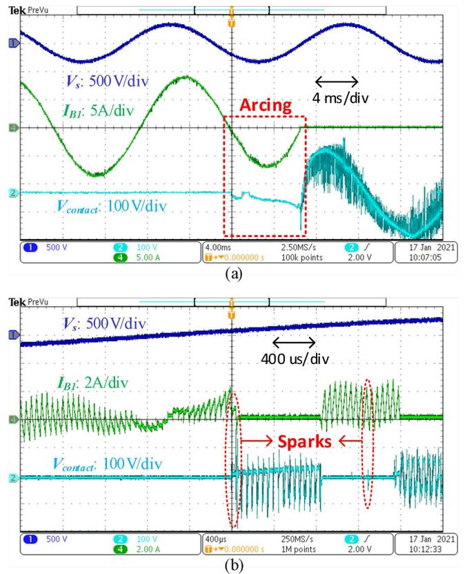
**FIGURE 18.** (a) Conventional SVR tap change waveform. (b) Arcless tap change waveform.
