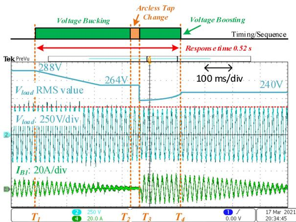
FIGURE 20. Prototype test waveforms of the collaborative operation.
