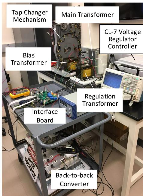
FIGURE 16. Proposed hybrid voltage regulator prototype.
