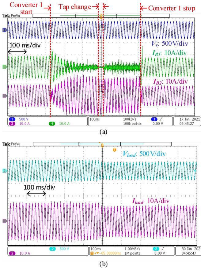
**FIGURE 17.** Arcless tap change waveforms. (a) Full operation process. (b) Load voltage and current waveform during the arcless tap change.
