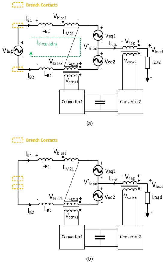
**FIGURE 4.** Equivalent circuits. (a) Bridging position. (b) Nonbridging position.
