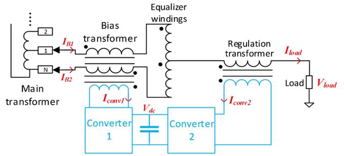
**FIGURE 3.** Proposed hybrid voltage regulator with a fractionally rated power converter.
