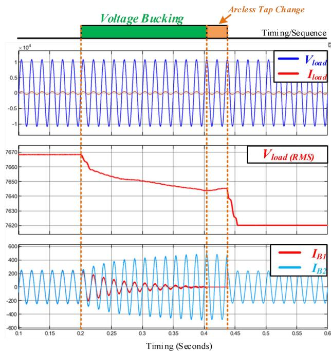
**FIGURE 13.** Collaborative operation simulation of power electronics voltage regulation and mechanical arcless tap change.
