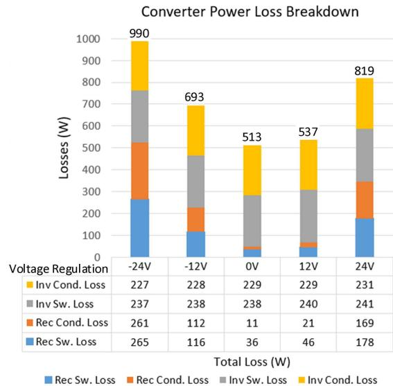
**FIGURE 14.** Converter power loss breakdown.
