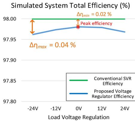
FIGURE 15. Simulated system total efficiency.
