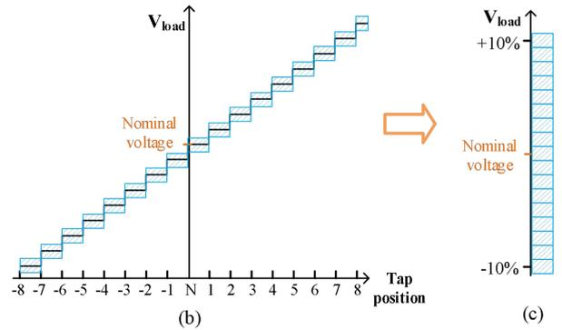
**FIGURE 7. Load voltage regulation principle for fixed source voltage  $V_s$ . (a) Conventional SVR with step voltage change. (b) Proposed hybrid voltage regulator with positive and negative half step voltage regulation range for each tap position. (c) Full range of the proposed stepless voltage regulation.**
