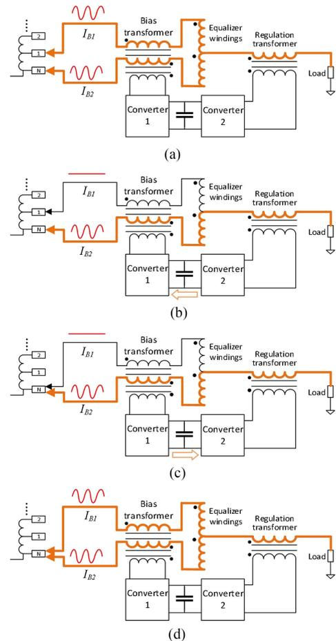
**FIGURE 5.** Arcless tap change operation sequence. (a) Converter 1 is disabled and Converter 2 regulates the dc bus voltage. (b) Upper branch current suppression. (c) Upper branch contact moves from tap 1 to tap  $N$ . (d) Converter 1 is shut down.
