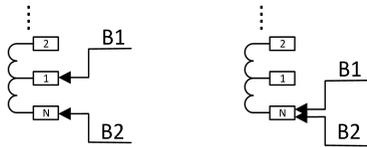
**FIGURE 2.** Bridging position (left) and nonbridging position (right).
