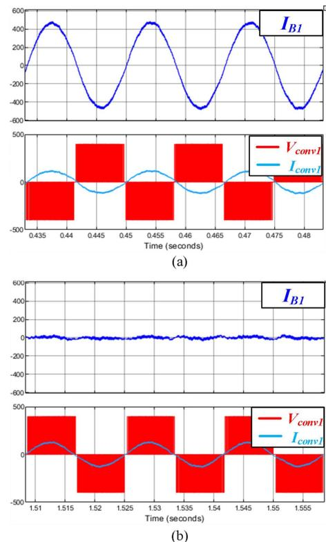
FIGURE 12. (a) Zoom-in waveforms before 0.5 s when Converter 1 is at maximum reverse power flow. (b) Zoom-in waveforms after 1.5 s when Converter 1 is at maximum forward power flow after 1.5 s.
