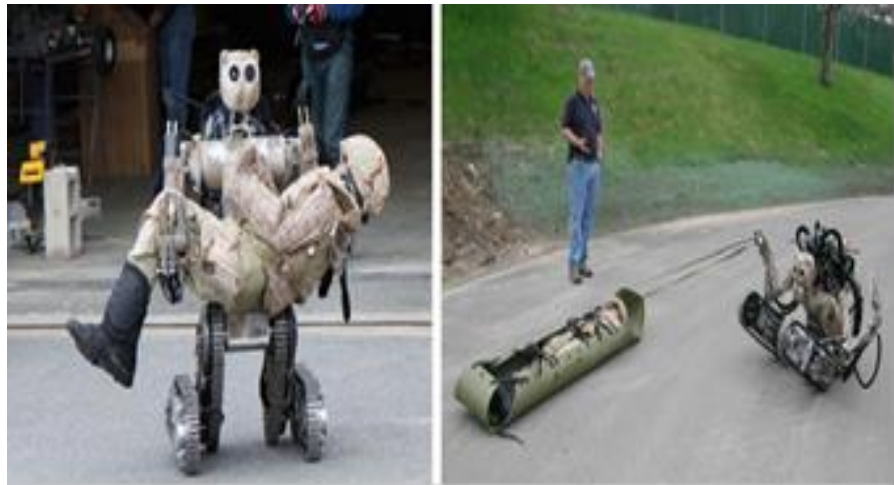
Figure 2.1.2.2 BEAR Robot used in the military for rescue operations [15]
