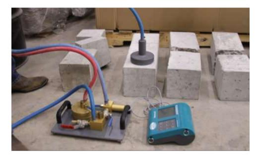
Figure 3.9: Torrent air permeability set up
