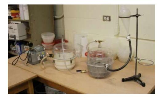
Figure 3.6: RCPT samples conditioning
