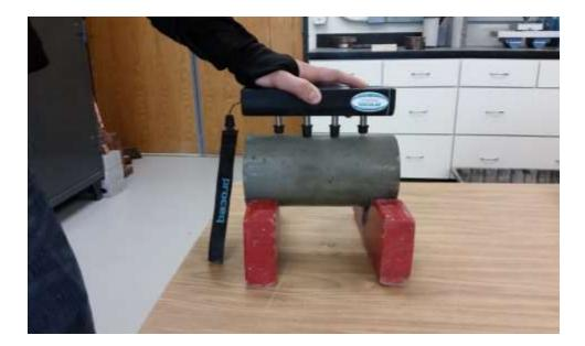
Figure 3.8: Surface resistivity Proceq set up
