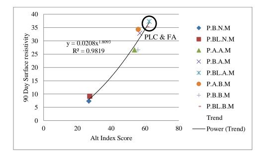
Figure 5.30: Alternative Index Score vs. 90 Day Surface Resistivity
