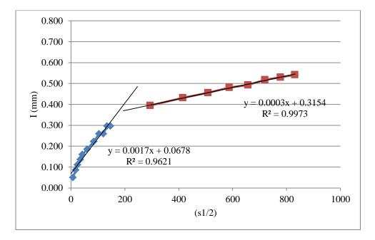
Figure 4.1: Example sorptivity graph (Sample P.B.B.M)
