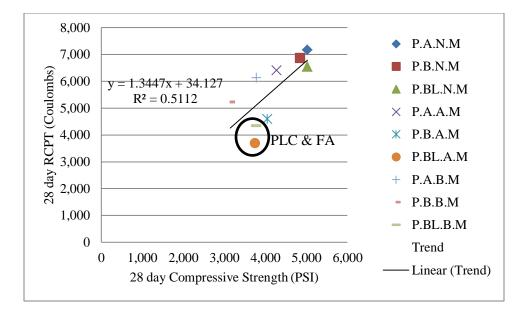
Figure 5.13: 28 day RCPT vs 28 day compressive strength
