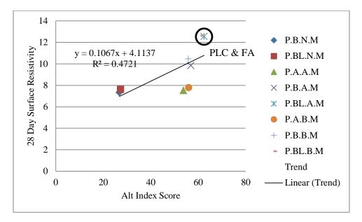
Figure 5.29: Alternative Index Score vs. 28 Day Surface Resistivity
