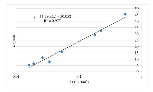
Figure 5.1: Air permeability Kt vs. L
