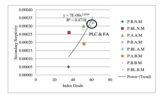
Figure 5.23: Secondary sorptivity vs. index grade
