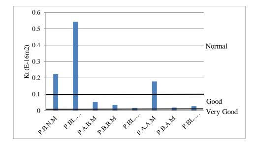
Figure 4.10: Air permeability results 4.4 Surface Resistivity Test Results
