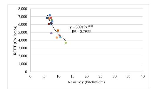
Figure 5.8: 28 day RCPT vs. surface resistivity
