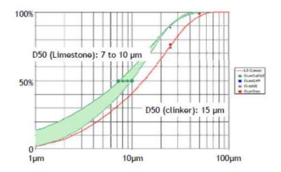
Figure 2.1: Limestone particle size distribution (Tennis et al., 2011)
