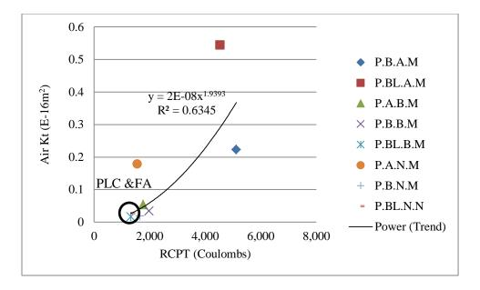
Figure 5.3: Air permeability vs. 90 day RCPT results
