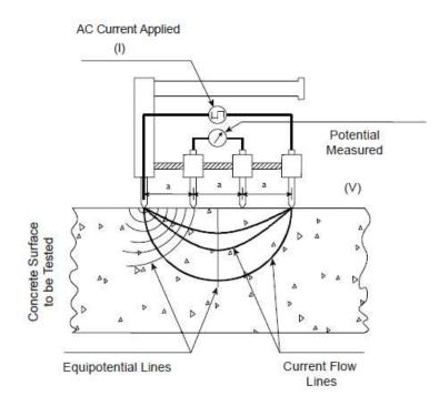
Figure 2.2: Four point Wenner array probe test set up (American Association of State Highway and Transportation Officials 2011)
