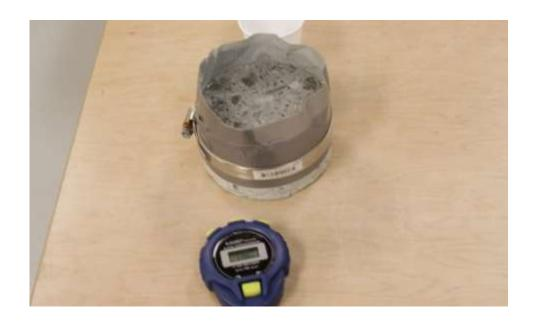
Figure 3.5 Ponding test set up
