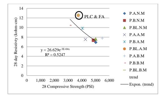
Figure 5.11: 28 day resistivity vs. 28 day compressive strength
