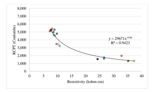
Figure 5.9: 90 Day RCPT vs. surface resistivity
