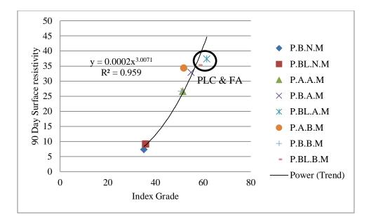
Figure 5.20: 90 day surface resistivity vs index grade
