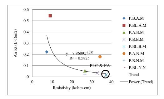
Figure 5.5: Air permeability vs. 90 day surface resistivity results
