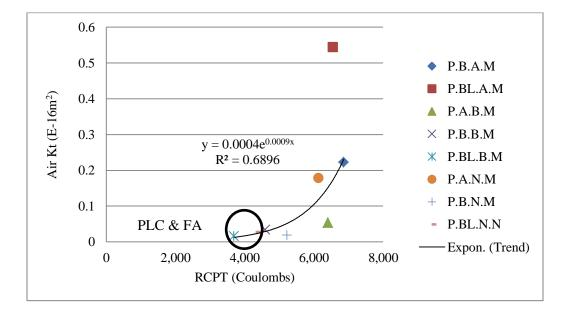
Figure 5.2: Air permeability vs. 28 day RCPT results
