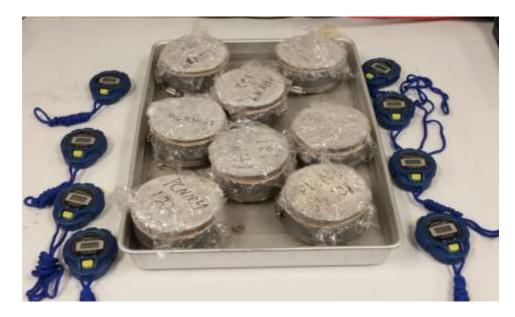
Figure 3.4: Suction method test set up
