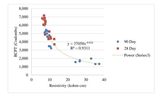
Figure 5.10: Combined RCPT vs. surface resistivity
