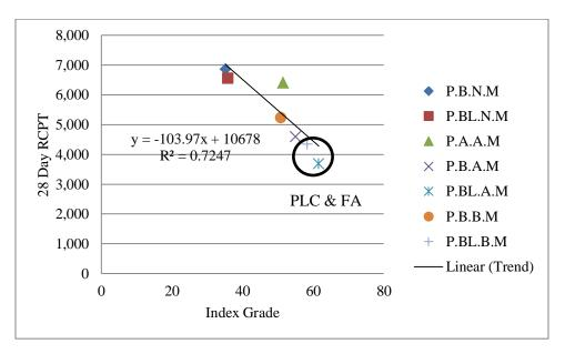
Figure 5.17: 28 day RCPT vs index grade
