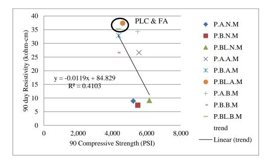
Figure 5.12: 90 day resistivity vs 90 day compressive strength
