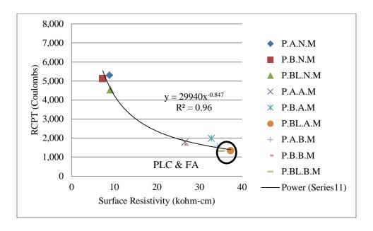
Figure 5.6: Select 28 day RCPT vs. surface resistivity
