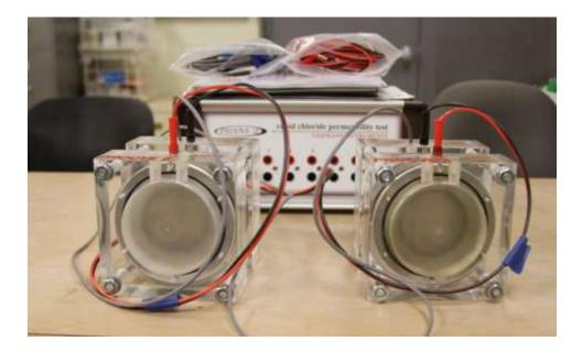
Figure 3.7: RCPT sample test set up
