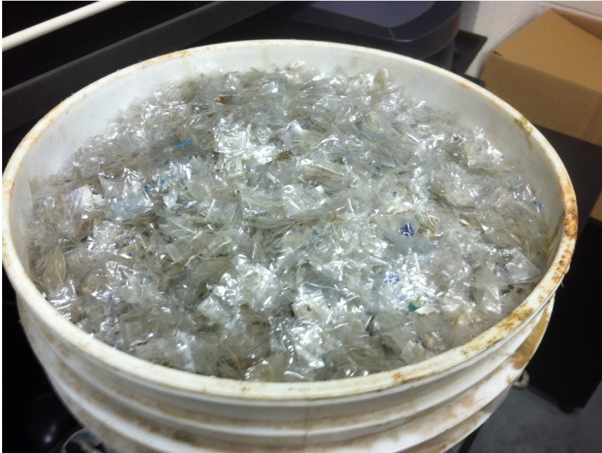
Figure 4.34: PET bale material processed in quantity for the preparation of triaxial test specimens
