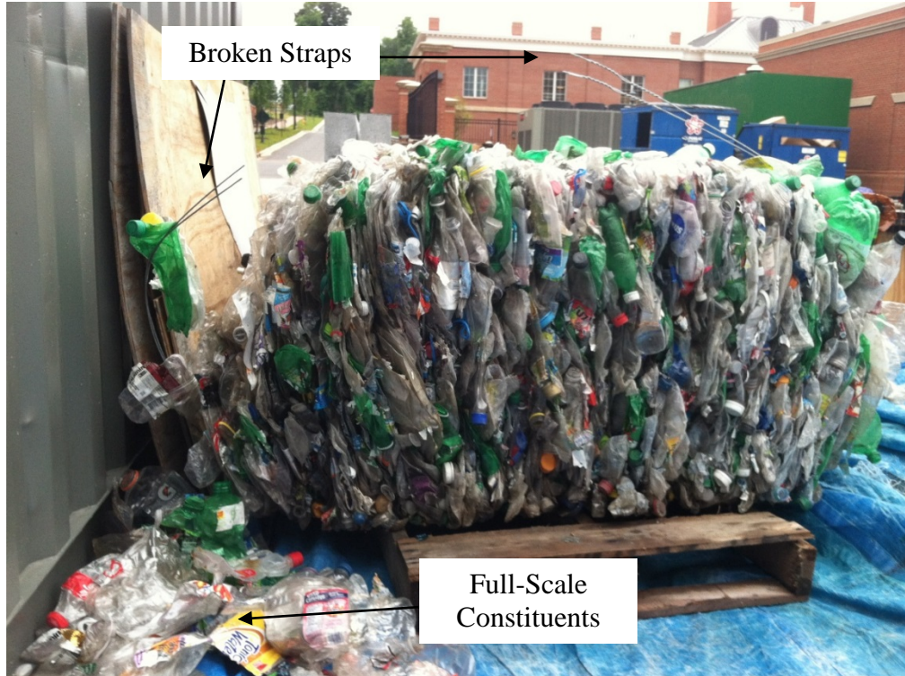
Figure 3.3: Recycled PET bale after the straps were cut
