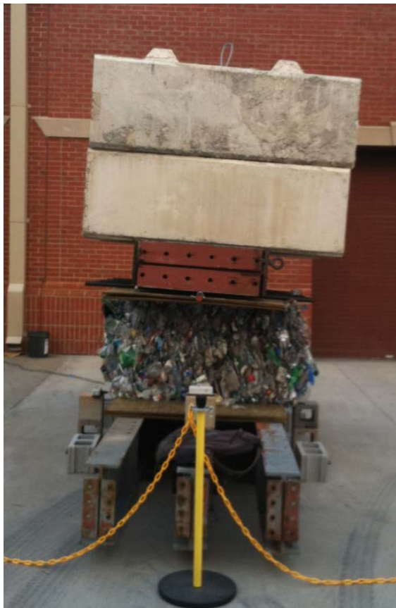
Figure 5.8: Photograph of the loaded PET test specimen exceeding a reasonable angle of inclination
