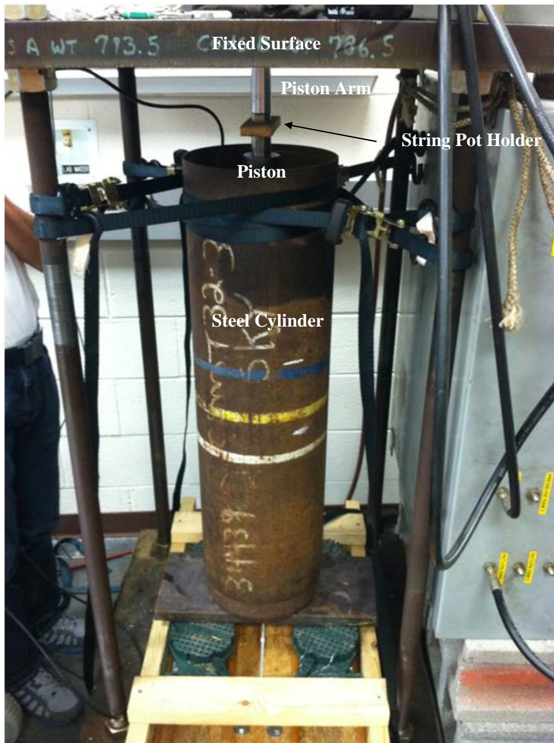
Figure 4.3: Photograph of the 22.86 cm inside diameter test configuration for the short-term, 1D compression test
