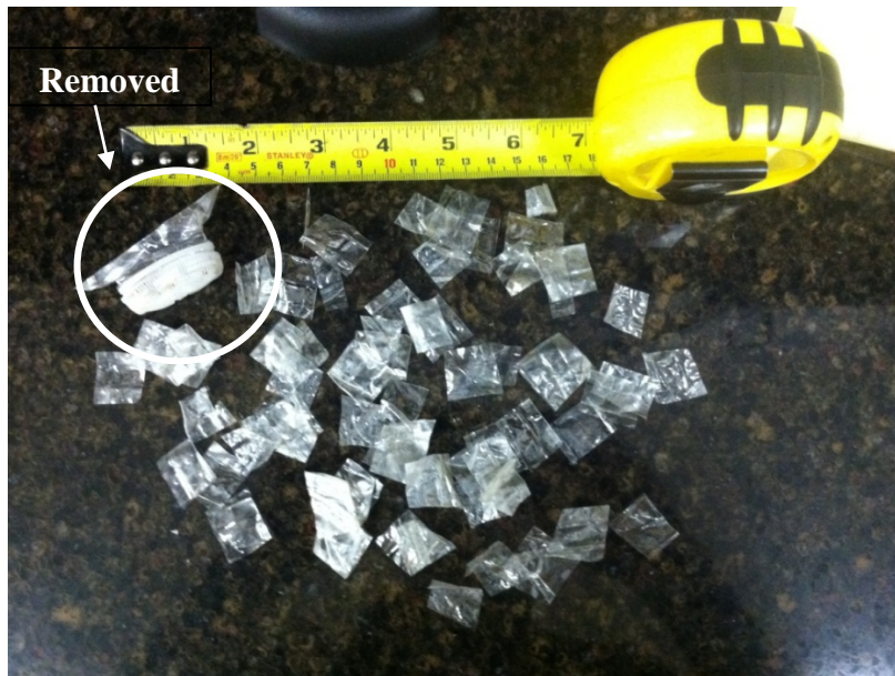
Figure 4.1: Chopped pieces of a Category 1 recycled PET bale constituent
