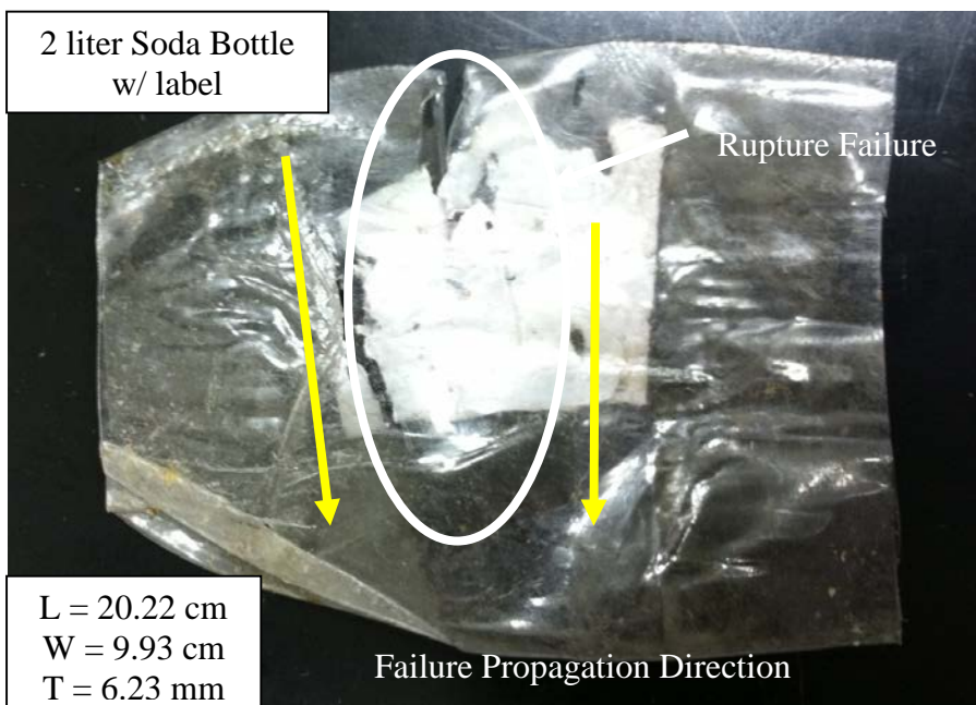
Figure 3.10: Post failure condition for Group 2 specimen
