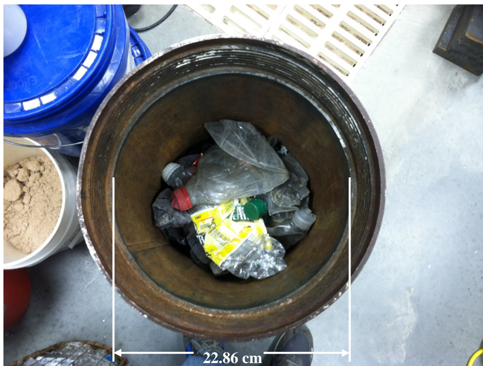
Figure 4.7: Photograph of the 22.86 cm diameter testing cylinder prior to 1D compression
